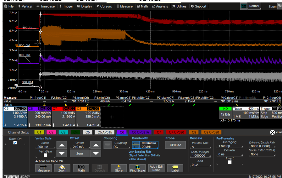
Figure 8-3. Driving four brushed-DC motors
