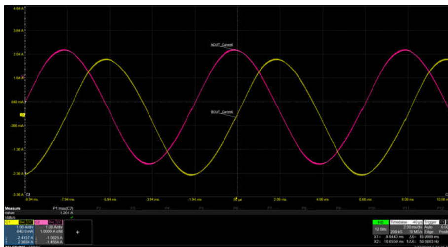
Figure 7-20. Coil Current Waveform with Silent Step Decay
