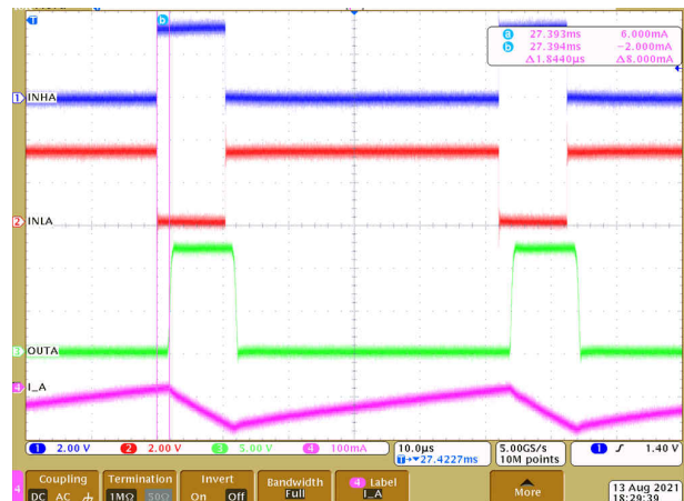
Figure 9-9. Driver delay compensation (1.8 \mu s)
