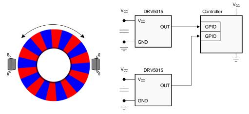
Figure 20. Incremental Rotary Encoding System
