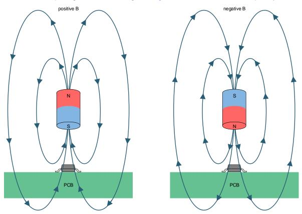
Figure 12. Flux Direction Polarity
