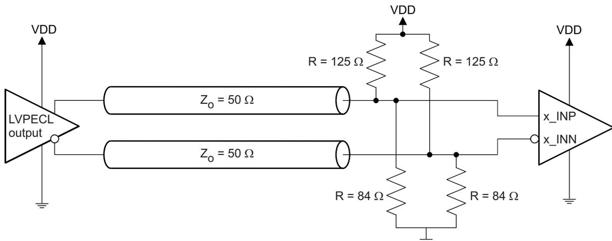
Figure 4. LVPECL Input Configuration During Device Test
