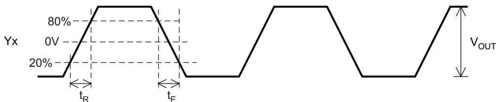
Figure 10. LVC1310 Output Voltage, and Rise and Fall Times
