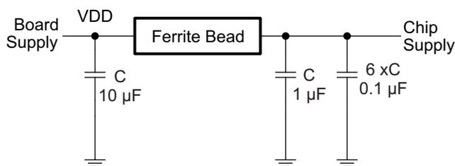
Figure 24. Power-Supply Decoupling
