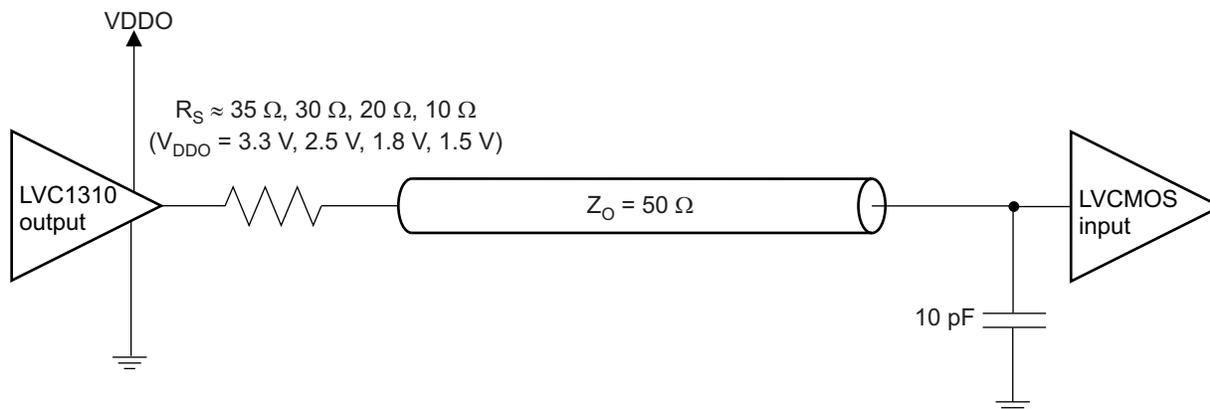
Figure 9. LVC1310 Output DC Configuration: Typical Application Load
