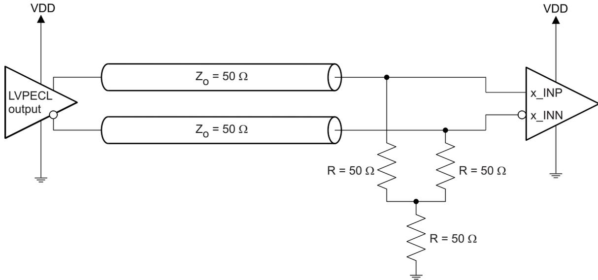
Figure 5. LVPECL Input Configuration During Device Test
