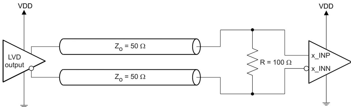
Figure 7. LVDS Input Configuration During Device Test
