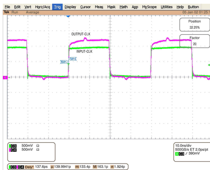
Figure 10-2. Input/Output Alignment in External Zero Delay Mode for LVCMOS Output
