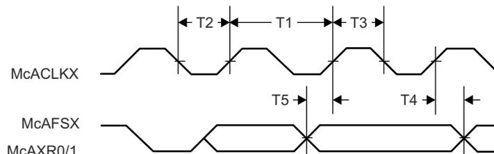
**Figure 7-16. I<sup>2</sup>S Receive Mode Timing Diagram**
