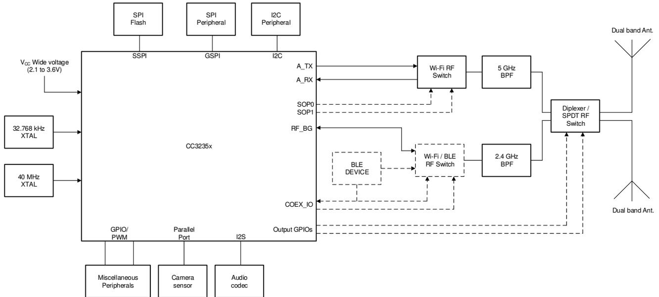
Note: The diplexer is used for the signal antenna solution. When using the antenna selection feature (dual antenna), an SPDT switch and two GPIO lines are required after the diplexer.
