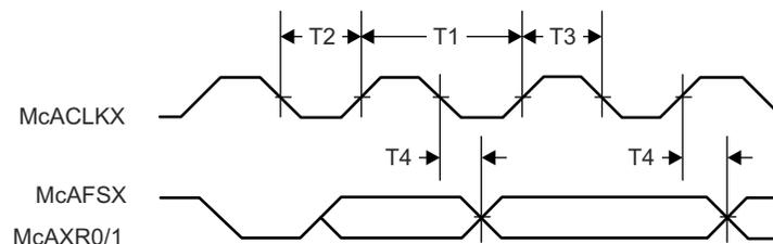
Figure 7-15. I<sup>2</sup>S Transmit Mode Timing Diagram
