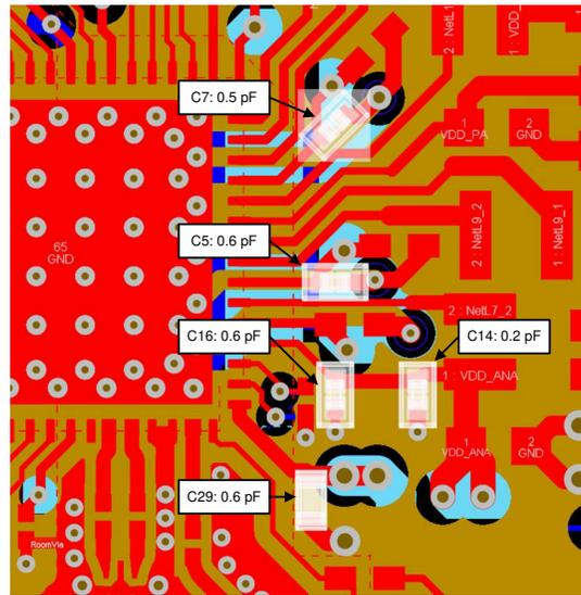
**Figure 9-9. Ground Routing for Input Decoupling Capacitors**
