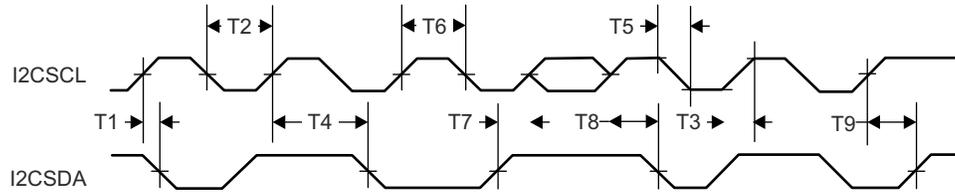
**Figure 7-18. I<sup>2</sup>C Timing Diagram**
