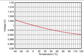
Figure 7-34. ADC Accuracy vs Temperature (V<sub>in</sub>=1V, Internal Reference, 200ksps)
