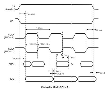
Figure 7-2. SPI Timing Diagram—Controller Mode, SPH = 1
