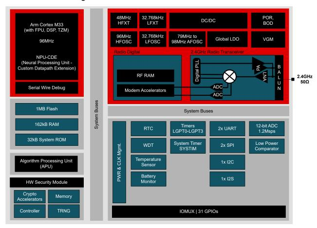
Figure 4-1. Functional Block Diagram
