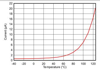
Figure 7-7. Standby Mode (MCU) Current vs Temperature (SRAM and partial register retention, RTC enabled), VDDS = 3.3V
