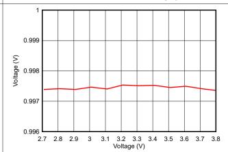
Figure 7-35. ADC Accuracy vs Supply Voltage (V<sub>in</sub>=1V, Internal Reference, 200ksps)
