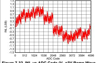
Figure 7-32. INL vs ADC Code (V<sub>in</sub>=3V Ramp Wave, Internal Reference, 200ksps)
