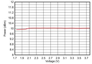
Figure 7-25. Ouput Power vs Supply Voltage (VDDS) (BLE 1Mbps, 2.44GHz, +10dBm)
