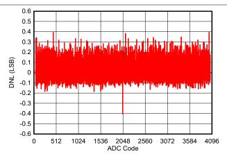
Figure 7-33. DNL vs ADC Code (V<sub>in</sub>=3V Sine Wave, Internal Reference, 200ksps)
