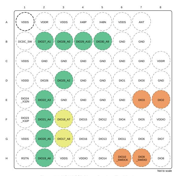
Figure 6-2. YCJ WCSP Pinout Preview (Top View)
