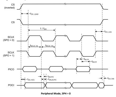
Figure 7-3. SPI Timing Diagram—Peripheral Mode, SPH = 0
