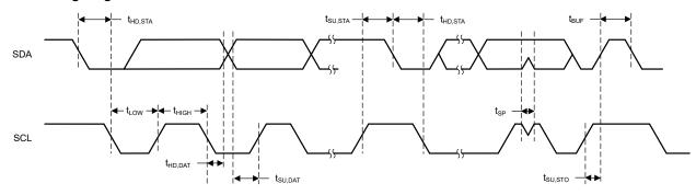
Figure 7-5. I<sup>2</sup>C Timing Diagram
