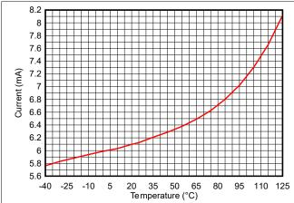
Figure 7-8. RX Current vs Temperature (BLE 1Mbps, 2.44GHz), VDDS = 3.3V
