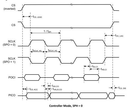
Figure 7-1. SPI Timing Diagram—Controller Mode, SPH = 0
