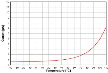
Figure 8-6. Standby Mode (MCU) Current vs. Temperature, 80kB RAM retention, no Cache retention, RTC On SCLK\_LF = 32 kHz XOSC, VDDS = 3.6 V
