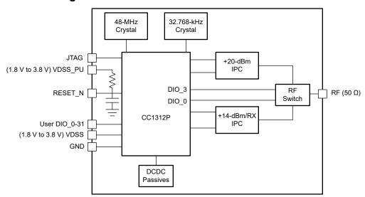
Figure 4-1. CC1312PSIP Block Diagram
