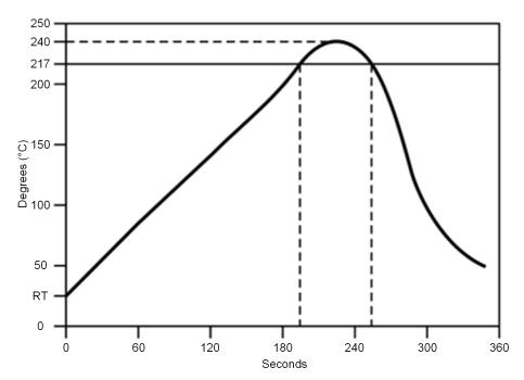
Figure 11-1. Temperature Profile for Evaluation of Solder Heat Resistance of a Component (at Solder Joint)
