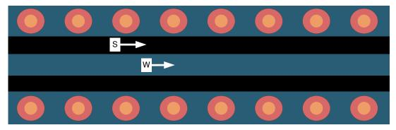
Figure 10-4. CPW With GND and Via Stitching (Top View)
