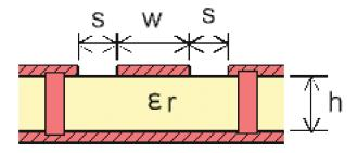
Figure 10-3. Coplanar Waveguide (Cross Section)
