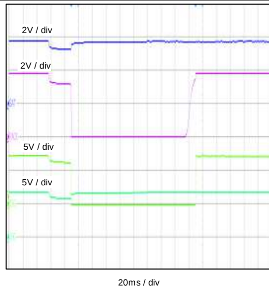
Figure 16. Overcurrent in Discharge Protection Set and Clear
