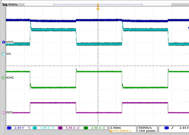
$V_{VBUS} = 5\text{ V}$                        $I_{INDPM} = 2\text{ A}$
