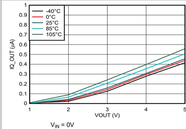
Figure 5-9. Output Quiescent Current vs Output Voltage
