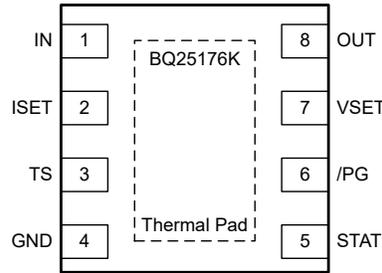
**Figure 4-1. DSG Package 8-Pin WSON Top View**
