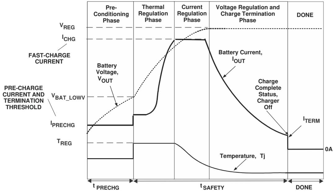
Figure 6-1. Lithium-Ion Battery Charging Profile with Thermal Regulation
