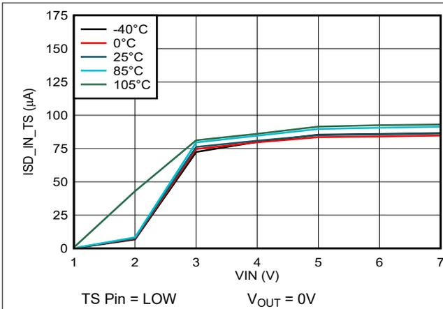
Figure 5-7. Input Shutdown Current vs Input Voltage
