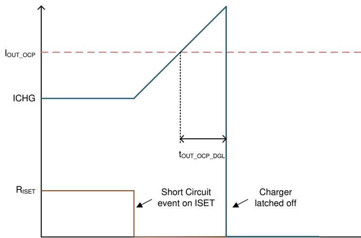
**Figure 6-4. Overcurrent Protection**
