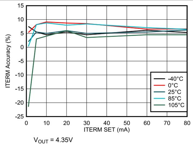
Figure 5-10. Termination Current Accuracy vs Termination Current Setting
