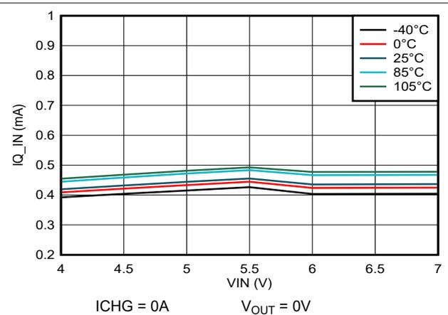
Figure 5-8. Input Quiescent Current vs Input Voltage
