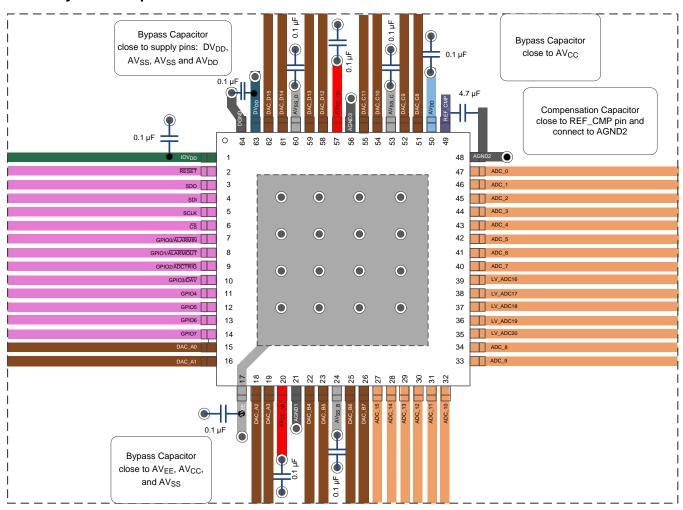
Figure 121. AMC7836 Example Board Layout
