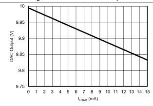
Figure 22. DAC Output Voltage vs Load Current
