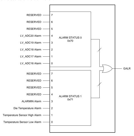
Figure 54. Alarm Status Register
