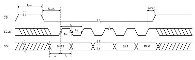
Figure 1. Serial Interface Write Timing Diagram
