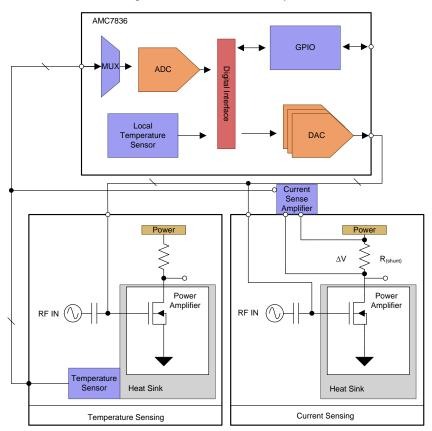
Figure 115. AMC7836 Example Control and Monitor System
