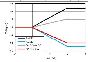
$AV_{SS} = AV_{EE} = -12 \text{ V}, AV_{CC} = 0 \text{ to } 12 \text{ V}, 2\text{-ms ramp}$
