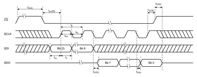
Figure 2. Serial Interface Read Timing Diagram
