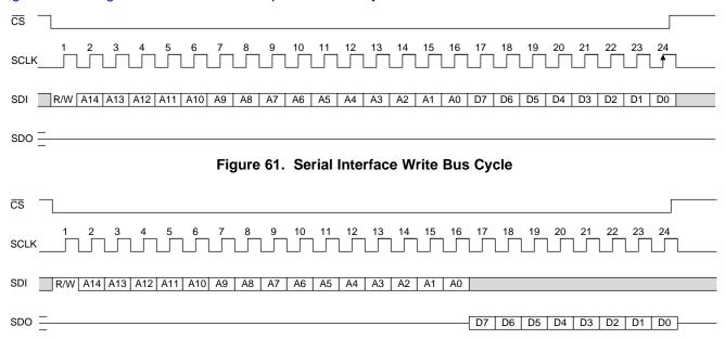
Figure 62. Serial Interface Read Bus Cycle
