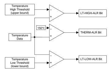
Figure 56. Internal Temperature Out-of-Range Alarms
