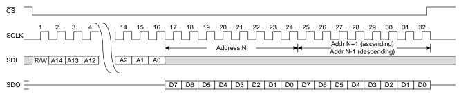
Figure 64. Serial Interface Streaming Read Example
