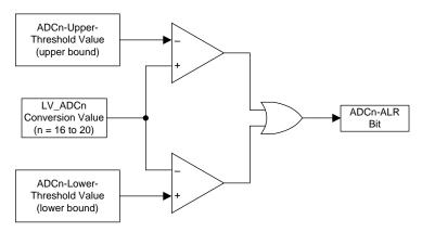
Figure 55. Unipolar Inputs Out-of-Range Alarms
