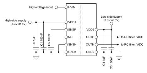
Figure 8-5. Decoupling of the AMC0381D-Q1
