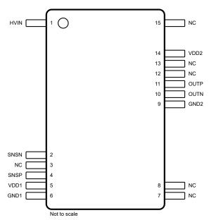
Figure 5-1. DFX Package, 15-Pin SOIC (Top View)
