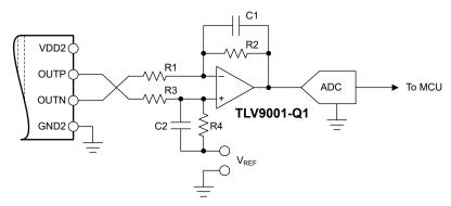
Figure 8-3. Connecting the AMC0381D-Q1 Output to a Single-Ended Input ADC
