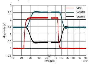
Figure 8-4. Step Response of the AMC0381D-Q1
