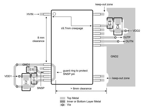
Figure 8-6. Recommended Layout of the AMC0381D-Q1
