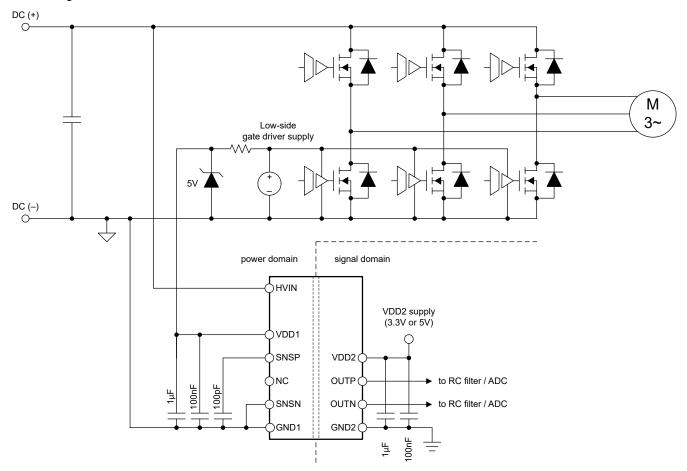
Figure 8-1. Using the AMC0381D-Q1 in a Typical Application
