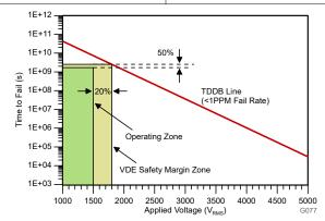
T<sub>A</sub> up to 150°C, stress-voltage frequency = 60Hz, isolation working voltage = 1500V<sub>RMS</sub>, projected operating lifetime ≥50 years
