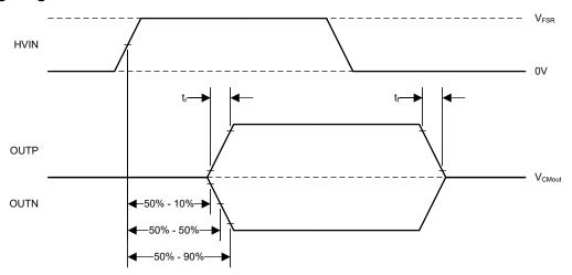
Figure 6-1. Rise, Fall, and Delay Time Definitions
