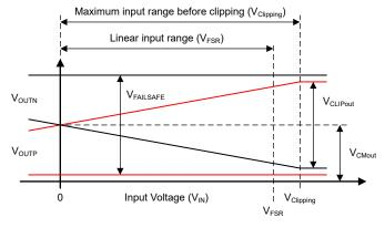
Figure 7-2. Input to Output Transfer Curve of the AMC0381D-Q1
