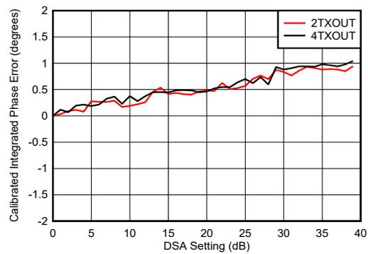
Integrated Phase Error =  $\text{Phase}(\text{DSA Setting}) - \text{Phase}(\text{DSA Setting} = 0)$
