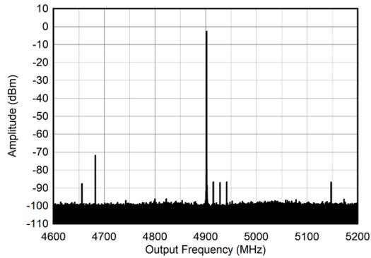
$f_{\text{DAC}} = 11796.48$  MSPS, interleave mode, 4.9 GHz matching, includes PCB and cable losses
