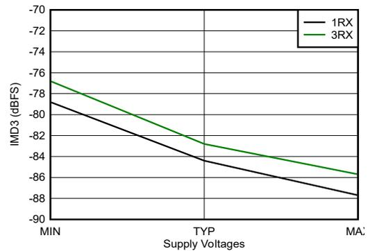
With 3.6 GHz matching,  $-7\text{ dBFS}$  each tone, 20-MHz tone spacing, all supplies at MIN, TYP, or MAX recommended operating voltages
