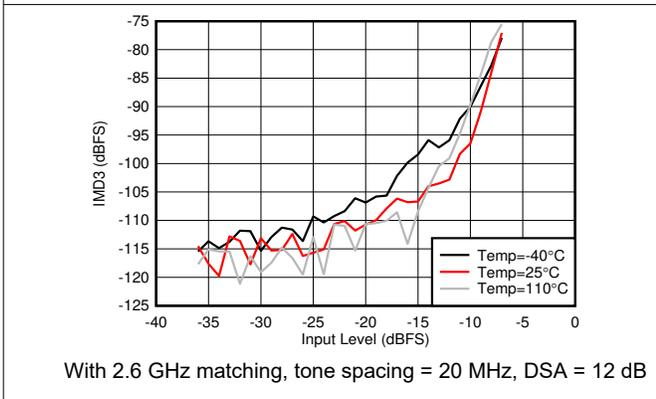
With 2.6 GHz matching, tone spacing = 20 MHz, DSA = 12 dB
