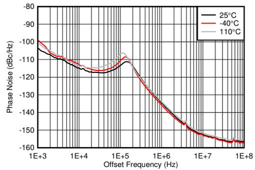
PLL enabled,  $f_{\text{VCO}} = 11796.48 \text{ MHz}$ ,  $f_{\text{REF}} = 491.52\text{MSPS}$ , measured at 2TXOUT
