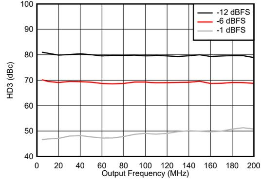
**Figure 4-258. HD3 vs Frequency 0 - 200 MHz**
