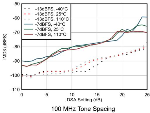
Figure 4-218. RX IMD3 vs DSA Setting at 6.851 GHz
