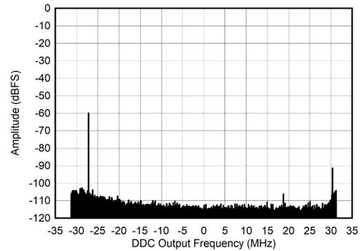
$A_{\text{IN}} = -60$  dBFS,  $f_{\text{ADC}} = 1500$  MSPS,  $f_{\text{NCO}} = 32.13$  MHz,
