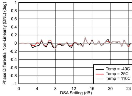
$$\text{Differential Phase Error} = \text{Phase}_{IN}(\text{DSA Setting} - 1) - \text{Phase}_{IN}(\text{DSA Setting})$$
