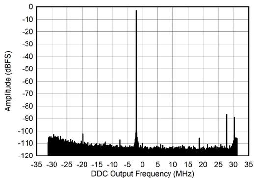
$A_{\text{IN}} = -3$  dBFS,  $f_{\text{ADC}} = 1500$  MSPS,  $f_{\text{NCO}} = 32.13$  MHz,
