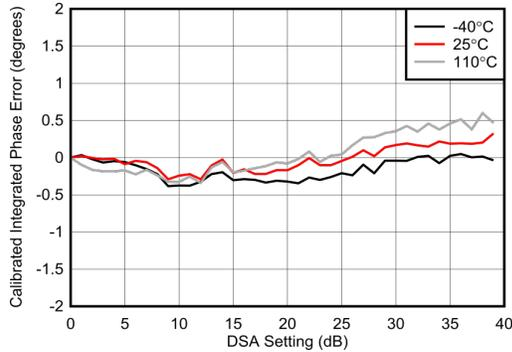
Integrated Phase Error = Phase(DSA Setting) – Phase(DSA Setting = 0)
