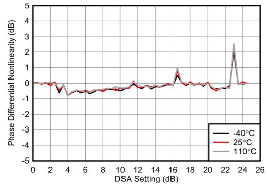
**Figure 4-207. RX Uncalibrated Differential Phase Error at 6.851 GHz**
