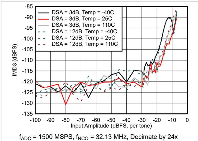
**Figure 4-23. IMD3 vs Input Amplitude at 30 MHz**
