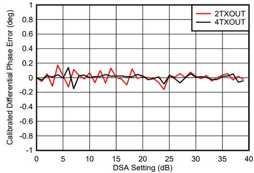
$f_{\text{DAC}} = 11796.48$  MSPS, interleaved mode, matching at 4.9 GHz
