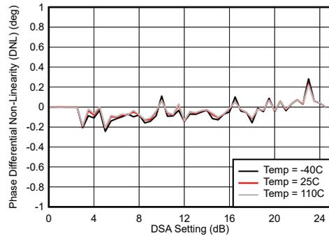
$$\text{Differential Phase Error} = \text{Phase}_{IN}(\text{DSA Setting} - 1) - \text{Phase}_{IN}(\text{DSA Setting})$$
