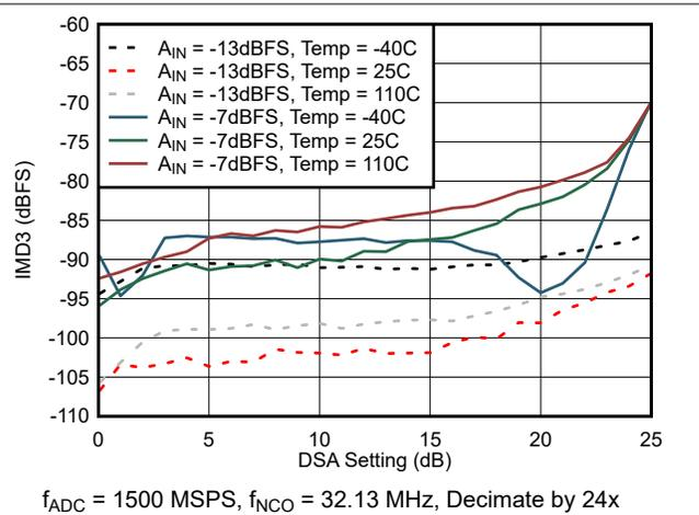
**Figure 4-24. IMD3 vs DSA Setting at 30 MHz**
