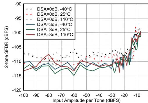
External clock mode, 50MHz tone spacing, excluding 3<sup>rd</sup> order distortion
