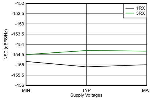
With 3.6 GHz matching, tone at -20 dBFS, 12.5-MHz offset frequency, all supplies at MIN, TYP, or MAX recommended operating voltages
