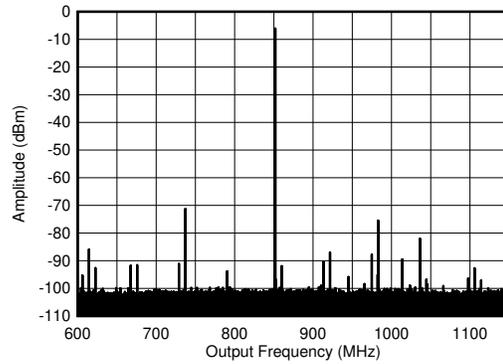
$f_{\text{DAC}} = 5898.24$  MSPS, straight mode, 0.8 GHz matching, includes PCB and cable losses
