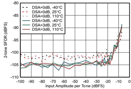
External clock mode, 20 MHz tone spacing, excluding 3<sup>rd</sup> order distortion
