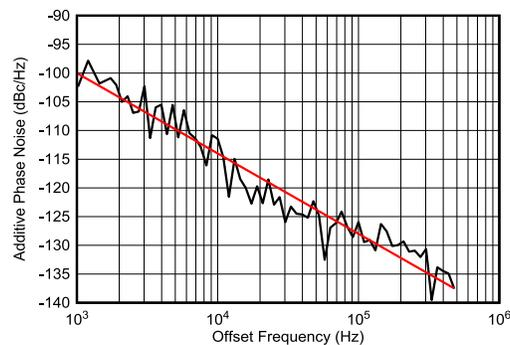
Figure 4-222. RX Additive Phase Noise at 6.85 GHz
