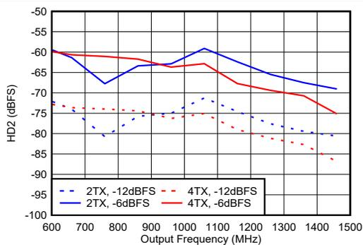
Matching at 0.8 GHz,  $f_{\text{DAC}} = 5898.24$  GSPS, straight mode
