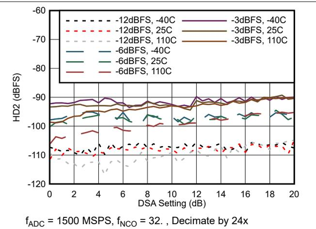
Figure 4-26. HD2 vs DSA Setting at 30 MHz
