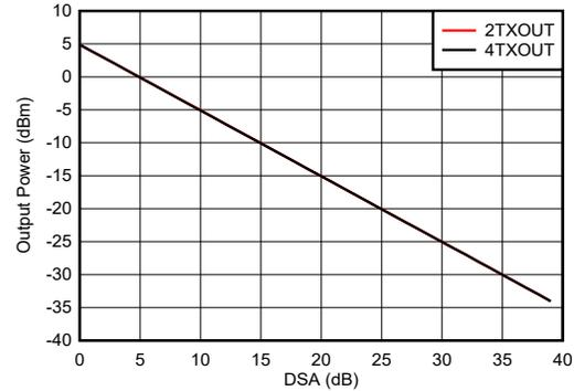
$f_{DAC} = 11796.48$  MSPS, interleaved mode,  $A_{out} = -0.5$  dBFS, matching 0.8 GHz
