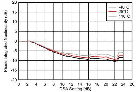
**Figure 4-209. RX Uncalibrated Integrated Phase Error at 6.851 GHz**
