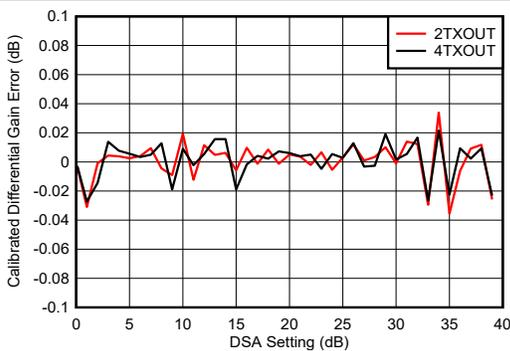
Differential Gain Error =  $\text{Gain}(\text{DSA Setting} - 1) - \text{Gain}(\text{DSA Setting})$
