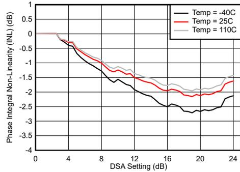
$$\text{Integrated Phase Error} = \text{Phase}(\text{DSA Setting}) - \text{Phase}(\text{DSA Setting} = 0)$$
