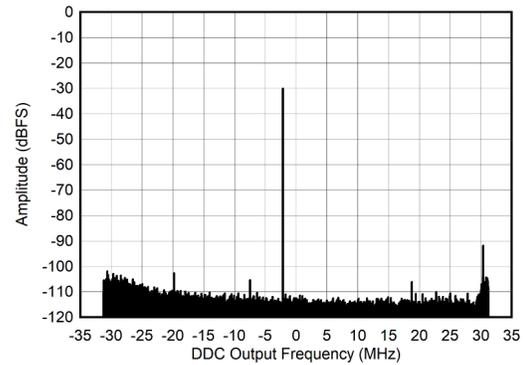
$A_{\text{IN}} = -30\text{ dBFS}$ ,  $f_{\text{ADC}} = 1500\text{ MSPS}$ ,  $f_{\text{NCO}} = 32.13\text{ MHz}$ ,
