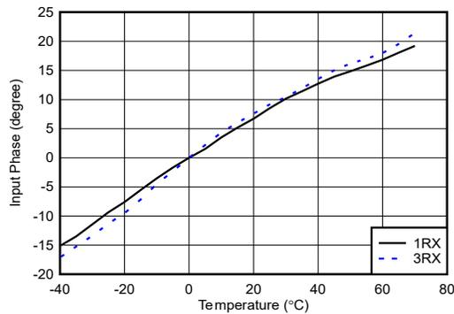
With 1.8 GHz matching, normalized to phase at  $25^\circ\text{C}$
