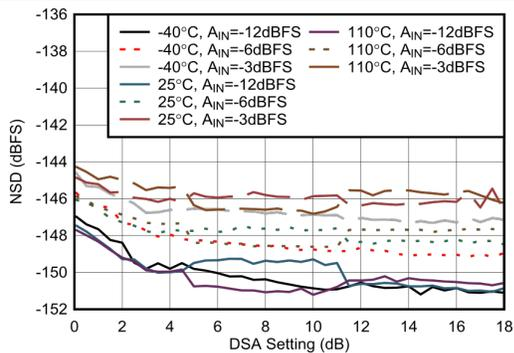
Figure 4-220. RX NSD vs DSA Setting at 6.851 GHz
