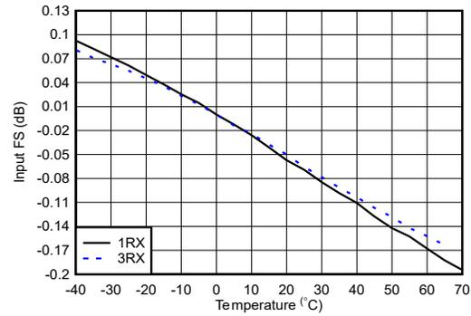
With 0.8 GHz matching, normalized to fullscale at  $25^\circ\text{C}$  for each channel
