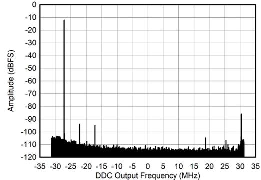
$A_{IN} = -12\text{ dBFS}$ ,  $f_{ADC} = 1500\text{ MSPS}$ ,  $f_{NCO} = 32.13\text{ MHz}$ ,
