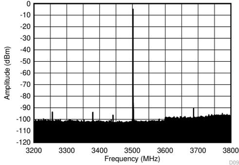
Matching at 3.5 GHz,  $f_{DAC} = 11.79648$  GSPS, interleave mode.
