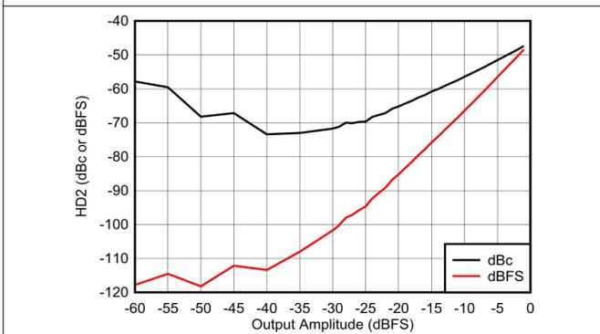
**Figure 4-291. HD2 vs Amplitude at 400 MHz**
