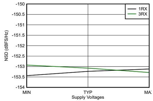
With 2.6 GHz matching, 12.5-MHz offset, all supplies at MIN, TYP, or MAX recommended operating voltages
