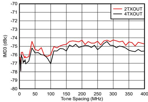
$f_{\text{DAC}} = 11796.48$  MSPS, interleaved mode, matching at 4.9 GHz,  $f_{\text{CENTER}} = 4.9\text{GHz}$ ,  $-13$  dBFS each tone
