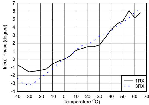
With 0.8 GHz matching, normalized to phase at  $25^\circ\text{C}$
