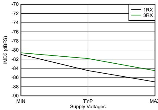
With 2.6 GHz matching,  $-7\text{ dBFS}$  each tone, 20-MHz tone spacing, all supplies at MIN, TYP, or MAX recommended operating voltages
