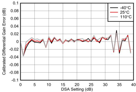
Differential Gain Error = Gain(DSA Setting – 1) – Gain(DSA Setting)
