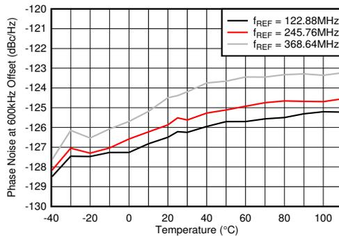
PLL enabled,  $f_{VCO} = 9830.4$  MHz, measured at 2TXOUT
