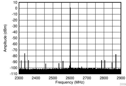
$f_{\text{DAC}} = 8847.36$  MSPS, straight mode, 2.6 GHz matching, includes PCB and cable losses
