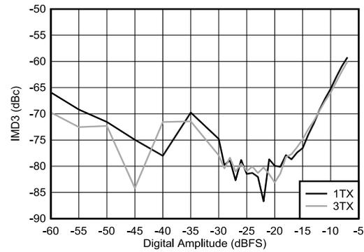
$f_{\text{DAC}} = f_{\text{CLK}} = 9000$  MSPS, non-interleave mode
