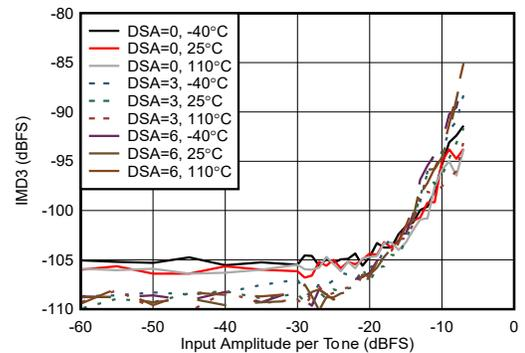
**Figure 4-217. RX IMD3 vs Input Amplitude at 6.851 GHz**
