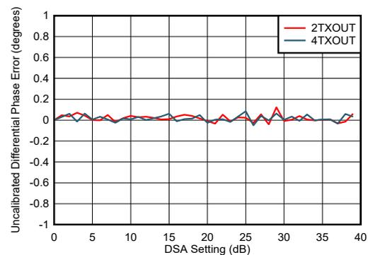
Differential Phase Error = Phase(DSA Setting – 1) – Phase(DSA Setting)
