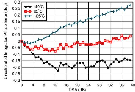
$f_{\text{DAC}} = 8847.36$  MSPS, straight mode, matching at 2.6 GHz, channel with the medium variation over DSA setting at 25°C
