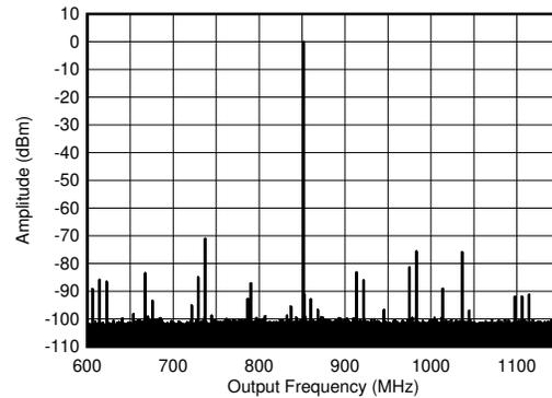
$f_{\text{DAC}} = 5898.24$  MSPS, straight mode, 0.8 GHz matching, includes PCB and cable losses
