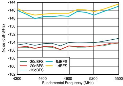
$f_{\text{DAC}} = 11796.48$  MSPS, interleave mode, matching at 4.9 GHz,  $A_{\text{out}} = -13$  dBFS.
