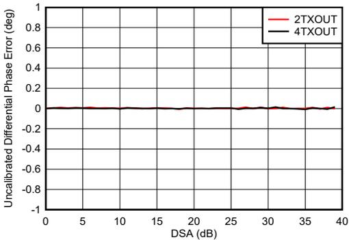
$f_{\text{DAC}} = 5898.24$  MSPS, interleave mode, matching at 0.8 GHz
