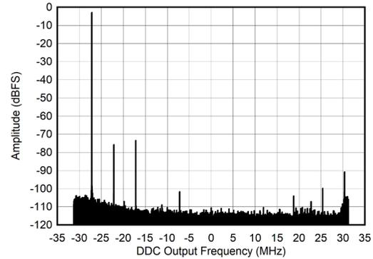
$A_{IN} = -3\text{ dBFS}$ ,  $f_{ADC} = 1500\text{ MSPS}$ ,  $f_{NCO} = 32.13\text{ MHz}$ ,
