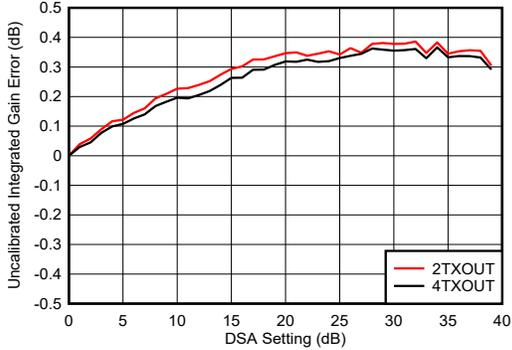
$f_{\text{DAC}} = 11796.48$  MSPS, interleave mode, matching at 4.9 GHz
