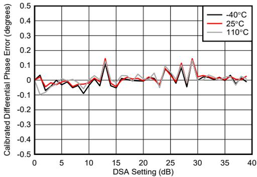
Differential Phase Error =  $\text{Phase}(\text{DSA Setting} - 1) - \text{Phase}(\text{DSA Setting})$
