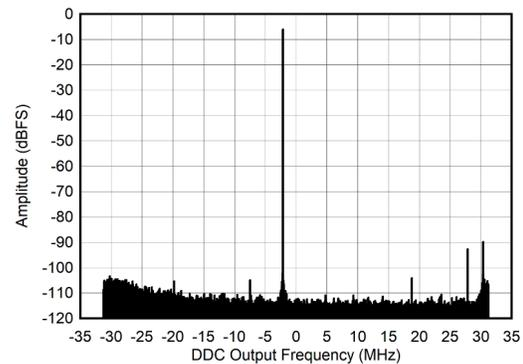
$A_{\text{IN}} = -6$  dBFS,  $f_{\text{ADC}} = 1500$  MSPS,  $f_{\text{NCO}} = 32.13$  MHz,
