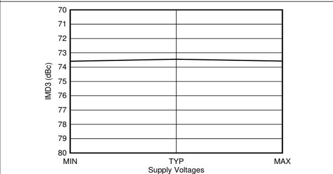
**Figure 4-435. TX IMD3 vs Supply Voltage at 2.6 GHz**
