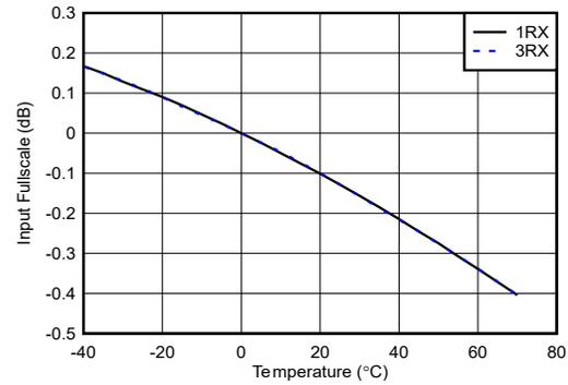
With 1.8 GHz matching, normalized to fullscale at  $25^\circ\text{C}$  for each channel
