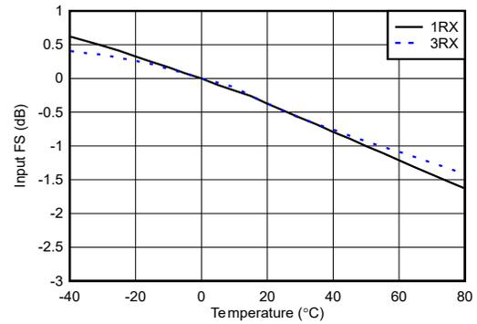
With 4.9 GHz matching, normalized to fullscale at  $25^\circ\text{C}$  for each channel
