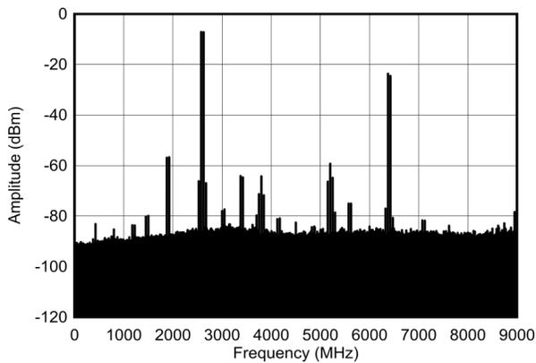
$f_{\text{DAC}} = 9000$  MSPS, external clock mode, non-interleave mode
