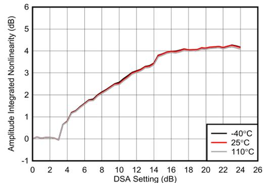
**Figure 4-205. RX Uncalibrated Integrated Amplitude Error at 6.851 GHz**
