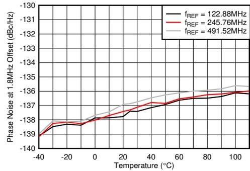
PLL enabled,  $f_{VCO} = 9830.4$  MHz, measured at 2TXOUT
