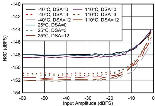
**Figure 4-216. RX NSD vs Input Amplitude at 6.851 GHz**
