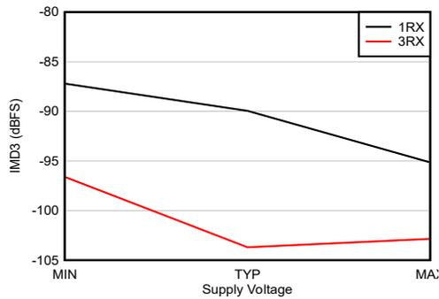
With 1.8 GHz matching, -7 dBFS each tone, 20-MHz tone spacing, all supplies at MIN, TYP, or MAX recommended operating voltages
