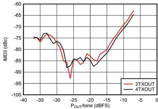
$f_{\text{DAC}} = 11796.48$  MSPS, interleaved mode, matching at 4.9 GHz,  $f_{\text{CENTER}} = 4.9\text{GHz}$ ,  $f_{\text{SPACING}} = 20$  MHz
