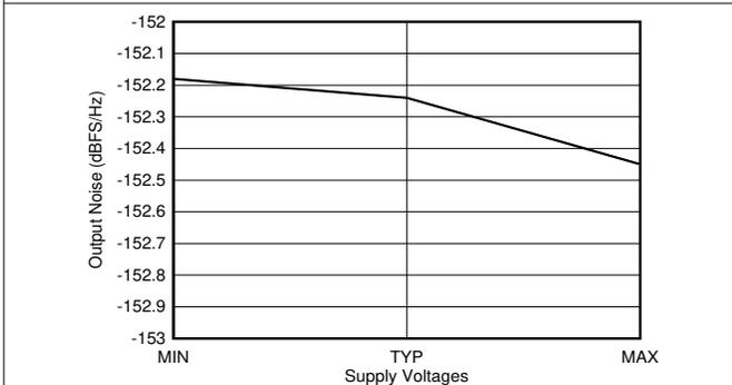
**Figure 4-434. TX Output Noise vs Supply Voltage at 2.6 GHz**
