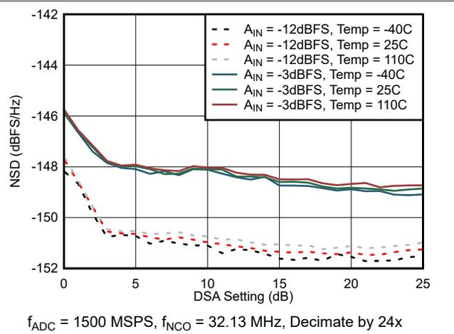
**Figure 4-22. NSD vs DSA Attenuation at 30 MHz**
