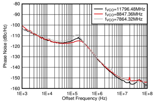
PLL enabled,  $f_{\text{REF}} = 491.52\text{MSPS}$ , measured at 2TXOUT
