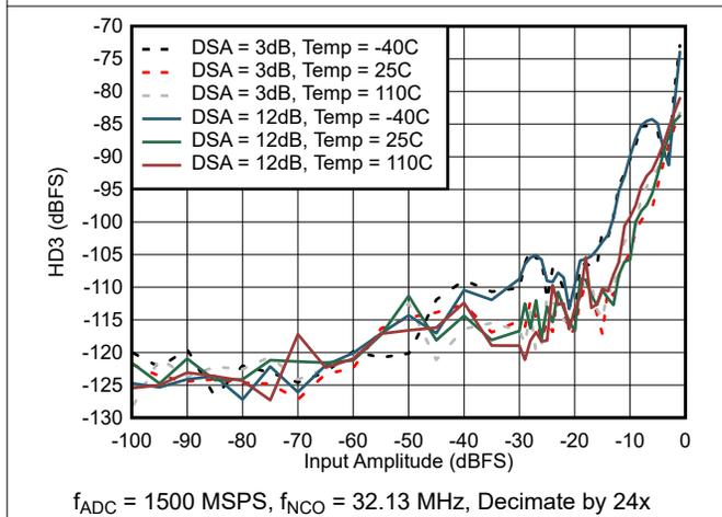
Figure 4-27. HD3 vs Input Amplitude at 30 MHz
