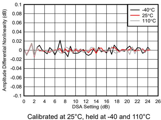
**Figure 4-204. RX Calibrated Differential Amplitude Error at 6.851 GHz**
