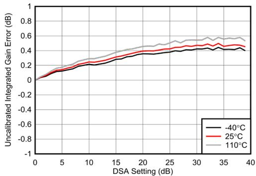
Integrated Gain Error = Gain(DSA Setting) – Gain(DSA Setting = 0).
