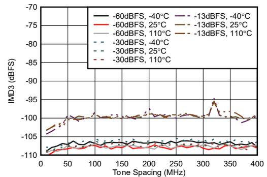
Figure 4-219. RX IMD3 vs Tone Spacing at 6.851 GHz
