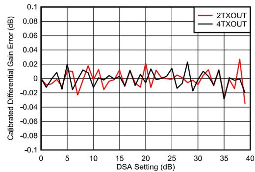
3.5 GHz Matching, included PCB and cable losses
