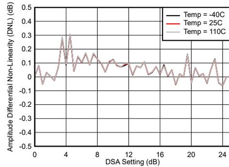
Differential Amplitude Error =  $P_{\text{IN}}(\text{DSA Setting} - 1) - P_{\text{IN}}(\text{DSA Setting}) + 1$
