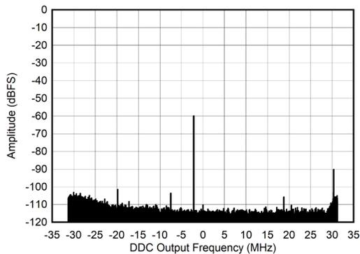
$A_{\text{IN}} = -60\text{ dBFS}$ ,  $f_{\text{ADC}} = 1500\text{ MSPS}$ ,  $f_{\text{NCO}} = 32.13\text{ MHz}$ ,
