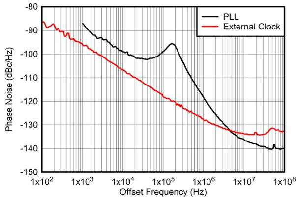
measured at TX output, normalized to 12GHz by  $20 \cdot \log_{10}(12\text{GHz}/F_{\text{OUT}})$
