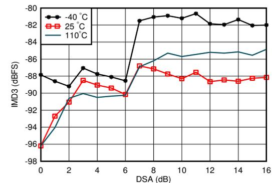
A. With 0.8 GHz matching, each tone  $-7 \text{ dBFS}$ , tone spacing = 20 MHz
