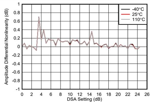
**Figure 4-203. RX Uncalibrated Differential Amplitude Error at 6.851 GHz**
