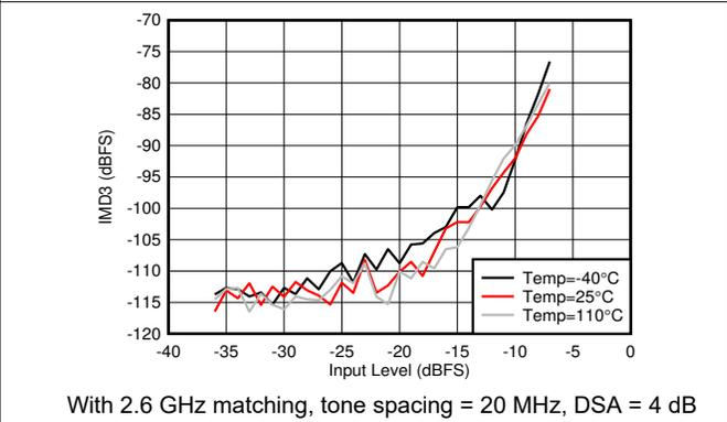
With 2.6 GHz matching, tone spacing = 20 MHz, DSA = 4 dB
