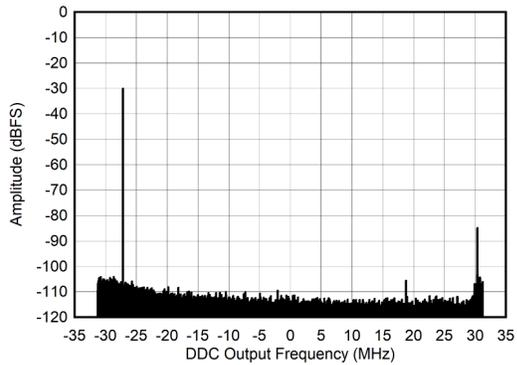
$A_{\text{IN}} = -30$  dBFS,  $f_{\text{ADC}} = 1500$  MSPS,  $f_{\text{NCO}} = 32.13$  MHz,
