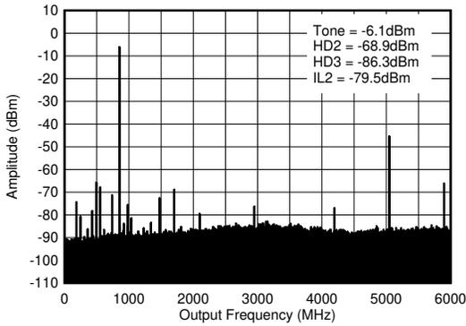
$f_{\text{DAC}} = 5898.24$ MSPS, straight mode, 0.8 GHz matching, includes PCB and cable losses.  $IL_n = f_s/n \pm f_{\text{OUT}}$  and is due to mixing with digital clocks.
