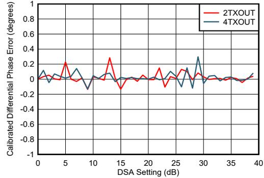
Differential Phase Error =  $\text{Phase}(\text{DSA Setting} - 1) - \text{Phase}(\text{DSA Setting})$
