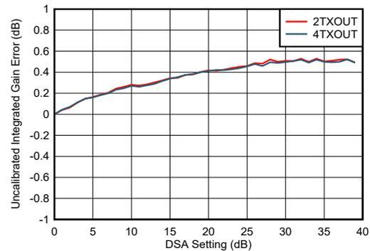
Integrated Gain Error = Gain(DSA Setting) – Gain(DSA Setting = 0).
