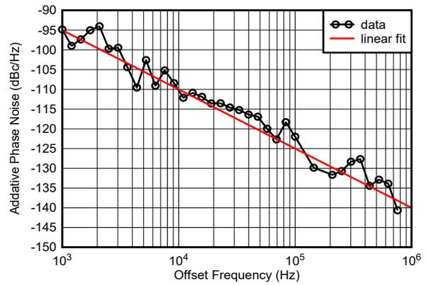
**Figure 4-591. RX Additive Phase Noise at 9.61GHz**
