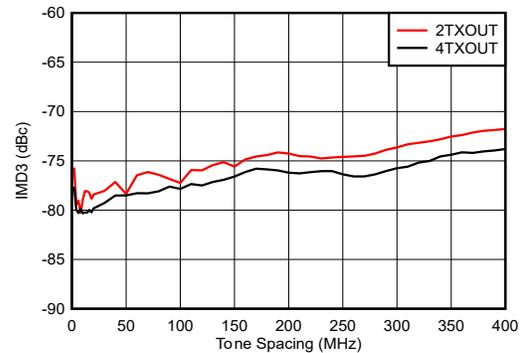
$f_{\text{DAC}} = 8847.36$  MSPS, straight mode,  $f_{\text{CENTER}} = 0.85$  GHz,
