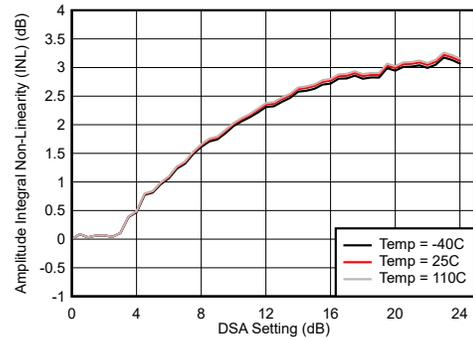
Integrated Amplitude Error =  $P_{\text{IN}}(\text{DSA Setting}) - P_{\text{IN}}(\text{DSA Setting} = 0) + (\text{DSA Setting})$
