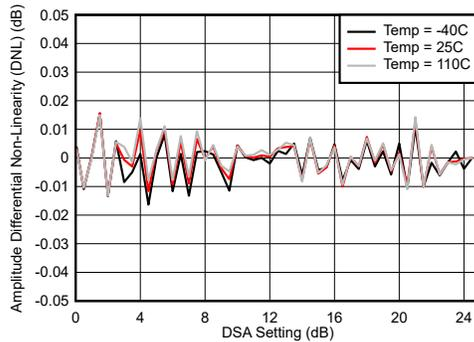
Differential Amplitude Error =  $P_{\text{IN}}(\text{DSA Setting} - 1) - P_{\text{IN}}(\text{DSA Setting}) + 1$
