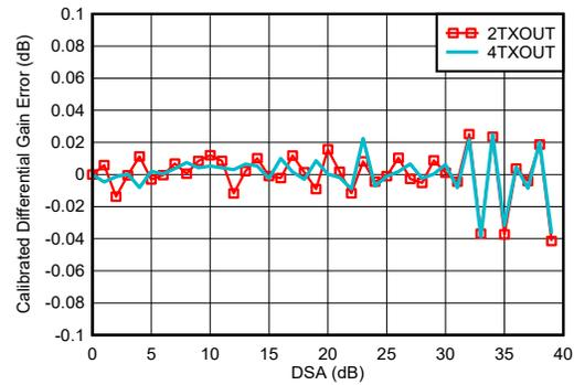
$f_{DAC} = 5898.24$  MSPS, interleaved mode, matching at 0.8 GHz
