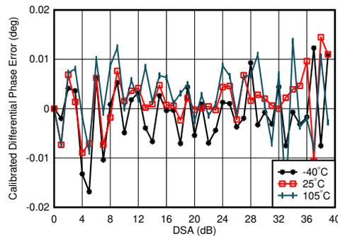
$f_{\text{DAC}} = 5898.24$  MSPS, interleave mode, matching at 0.8 GHz, channel with the median variation over DSA setting at 25°C
