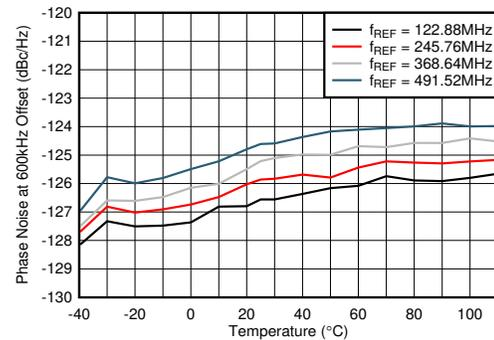
PLL enabled,  $f_{VCO} = 11796.48$  MHz, measured at 2TXOUT
