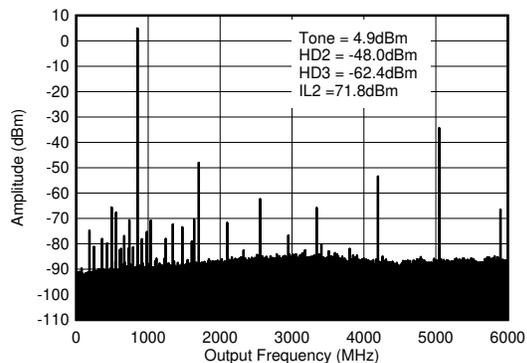
$f_{\text{DAC}} = 5898.24$  MSPS, straight mode, 0.8 GHz matching, includes PCB and cable losses.  $\text{IL}_n = f_s/n \pm f_{\text{OUT}}$  and is due to mixing with digital clocks.
