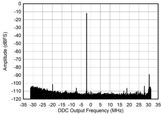
$A_{\text{IN}} = -12\text{ dBFS}$ ,  $f_{\text{ADC}} = 1500\text{ MSPS}$ ,  $f_{\text{NCO}} = 32.13\text{ MHz}$ ,
