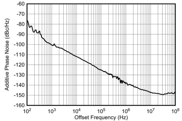
**Figure 4-589. External Clock Additive Phase Noise at 7.1 GHz**
