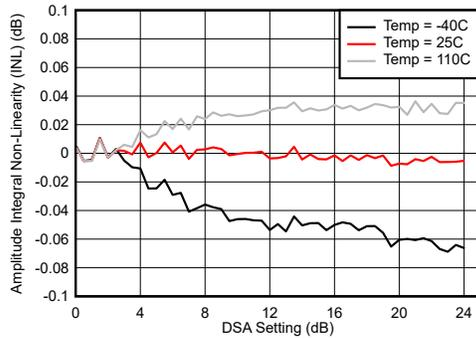
$$\text{Integrated Amplitude Error} = P_{IN}(\text{DSA Setting}) - P_{IN}(\text{DSA Setting} = 0) + (\text{DSA Setting})$$
