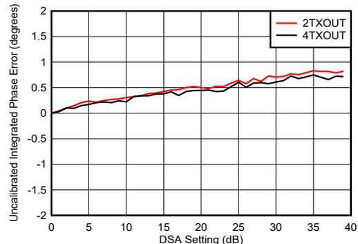
Integrated Phase Error =  $\text{Phase}(\text{DSA Setting}) - \text{Phase}(\text{DSA Setting} = 0)$
