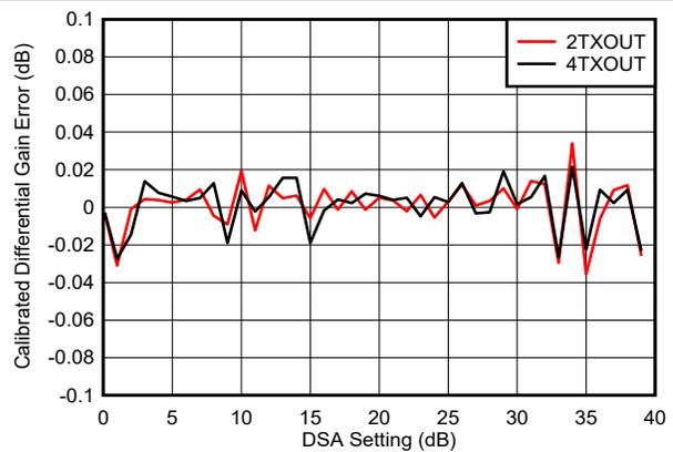
Differential Gain Error =  $\text{Gain}(\text{DSA Setting} - 1) - \text{Gain}(\text{DSA Setting})$
