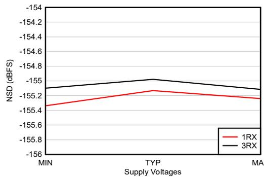
With 0.8 GHz matching, 12.5-MHz offset, all supplies at MIN, TYP, or MAX recommended operating voltages
