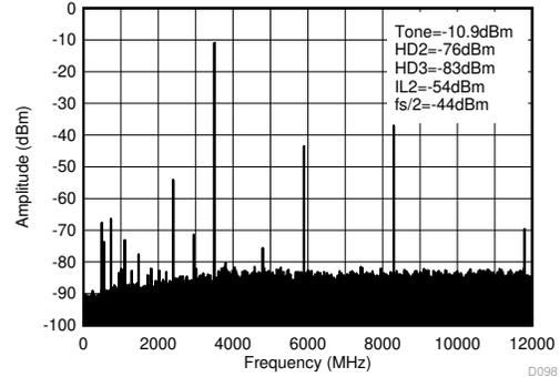
Matching at 3.5 GHz,  $f_{DAC} = 11.79648$  GSPS, interleave mode.
