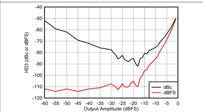
**Figure 4-292. HD3 vs Amplitude at 400 MHz**
