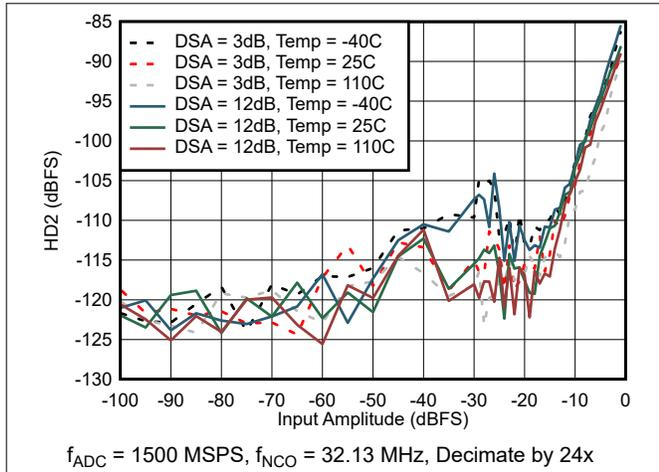
Figure 4-25. HD2 vs Input Amplitude at 30 MHz
