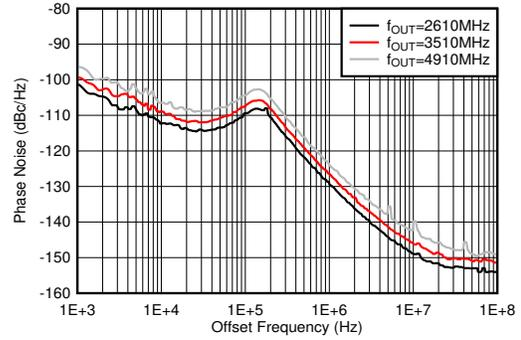
PLL enabled,  $f_{VCO} = 8847.36$  MHz,  $f_{REF} = 491.52$  MSPS, measured at 2TXOUT
