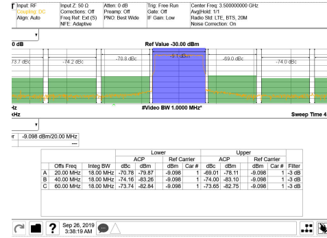
Figure 5-480. TX 20-MHz LTE Output Spectrum at 3.5 GHz (Band 42)
