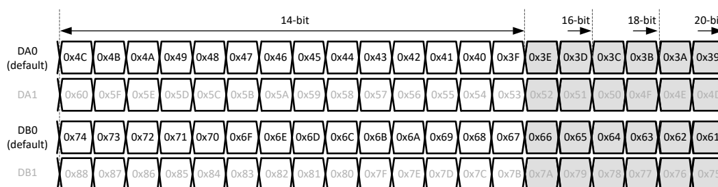
Figure 8-44. 1-wire output bit mapping
