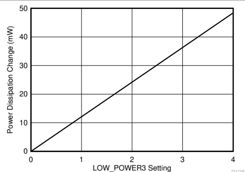
Figure 6-13. Power Dissipation Change vs LOW_POWER3 register setting
