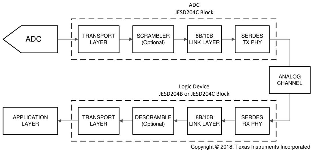
**Figure 6-5. Simplified 8B/10B Encoded JESD204C Interface Diagram**
