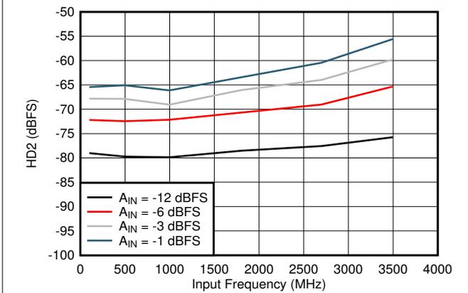
Figure 5-21. HD2 vs Input Frequency
