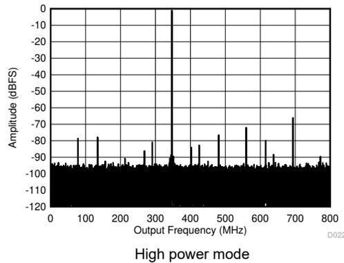
**Figure 5-4. Single Tone FFT at 347 MHz and -1 dBFS**
