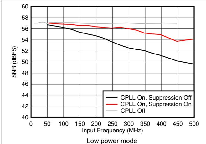
Figure 5-45. SNR vs  $F_{IN}$  and C-PLL modes
