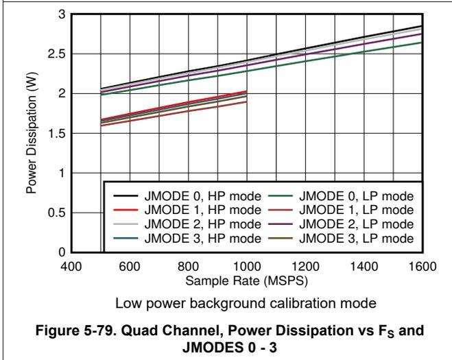
Figure 5-79. Quad Channel, Power Dissipation vs  $F_S$  and JMODES 0 - 3
