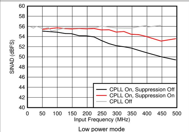
Figure 5-46. SINAD vs  $F_{IN}$  and C-PLL modes
