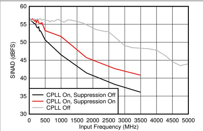
Figure 5-42. SINAD vs  $F_{IN}$  and C-PLL modes
