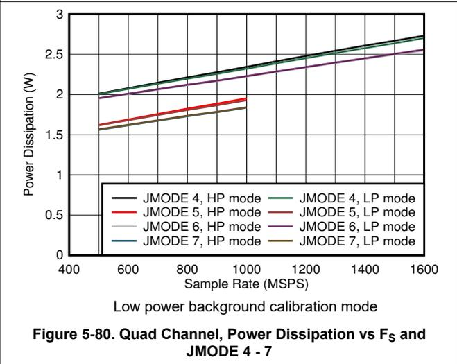
Figure 5-80. Quad Channel, Power Dissipation vs  $F_S$  and JMODE 4 - 7
