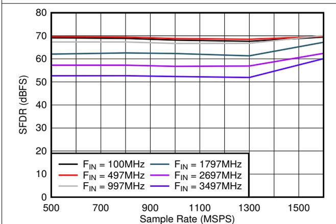
Figure 5-23. SFDR vs Sample Rate
