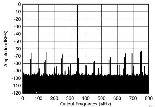
**Figure 5-6. Single Tone FFT at 347 MHz and -1 dBFS**
