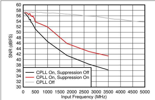
Figure 5-41. SNR vs  $F_{IN}$  and C-PLL modes
