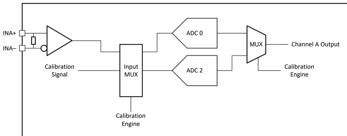
**Figure 6-15. Single Channel Calibration System Block Diagram**
