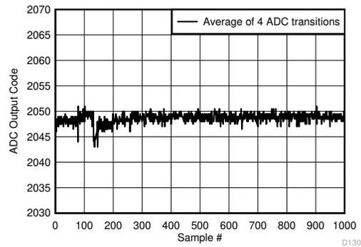
BG Calibration, midscale input voltage,  $ADC\_SRC\_DLY=31$ ,  $MUX\_DLY=30$
