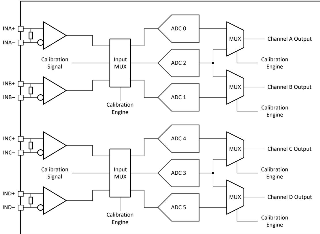
**Figure 6-13. Quad Channel Calibration System Block Diagram**
