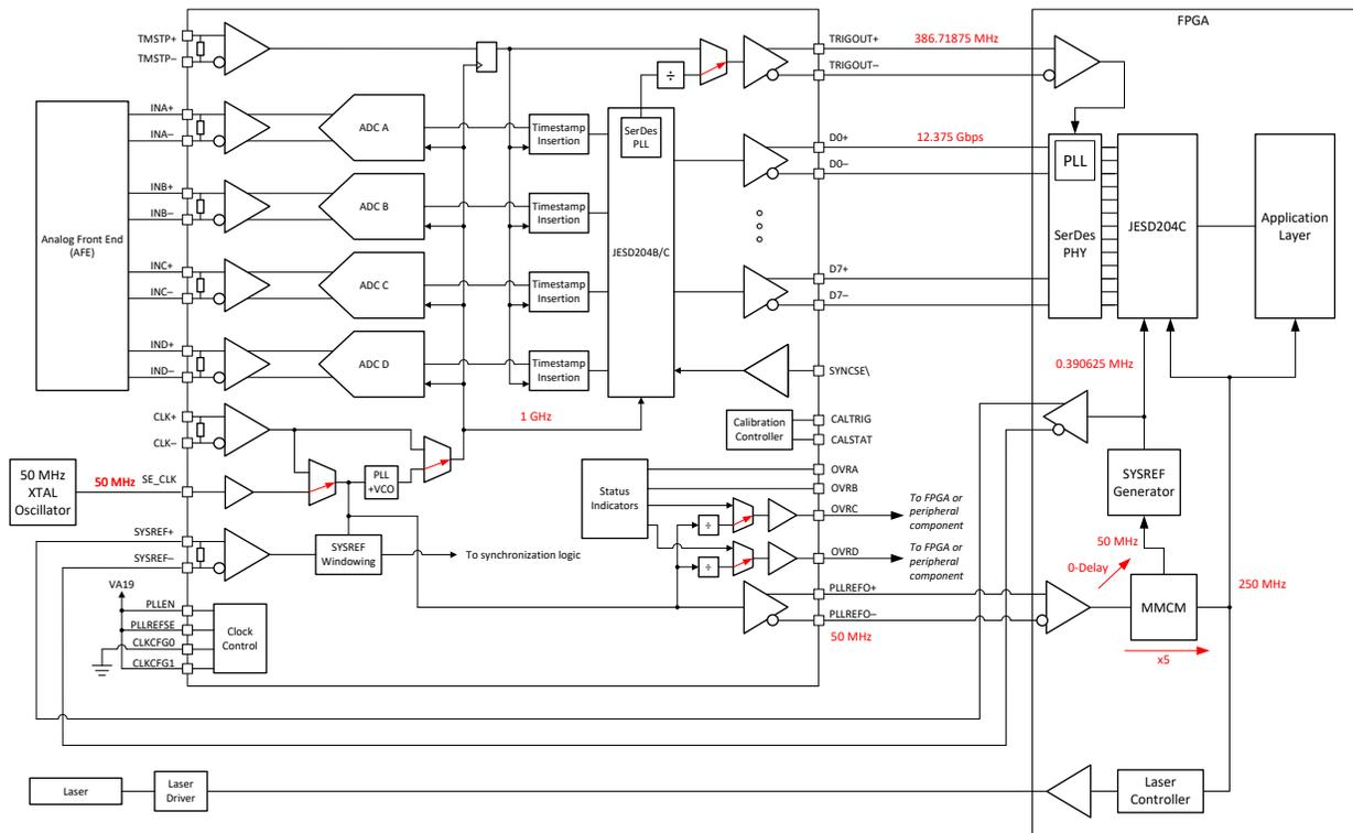
Figure 7-1. Typical Configuration for a LiDAR Digitizer
