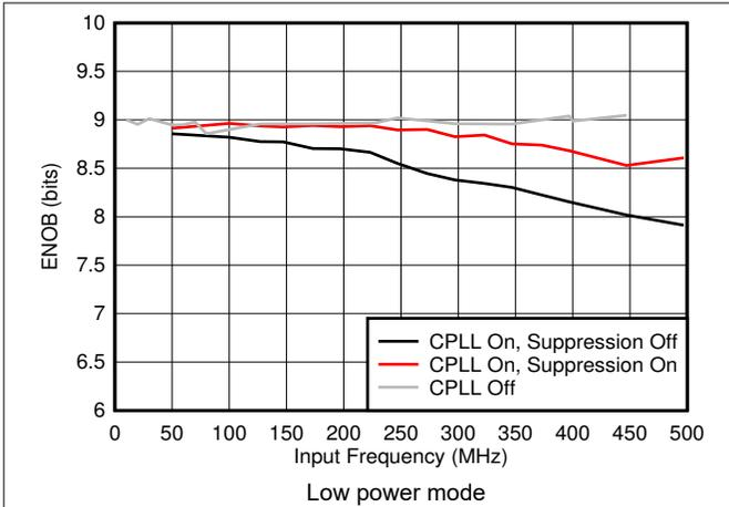
Figure 5-47. ENOB vs  $F_{IN}$  and C-PLL modes
