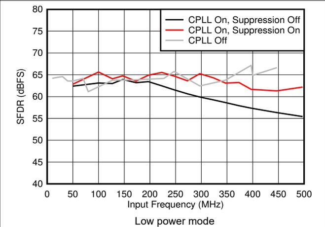
Figure 5-44. SFDR vs  $F_{IN}$  and C-PLL modes
