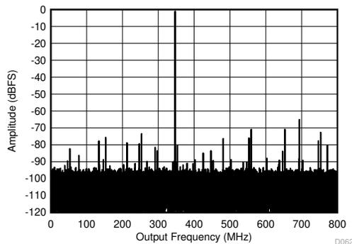
**Figure 5-5. Single Tone FFT at 347 MHz and -1 dBFS**
