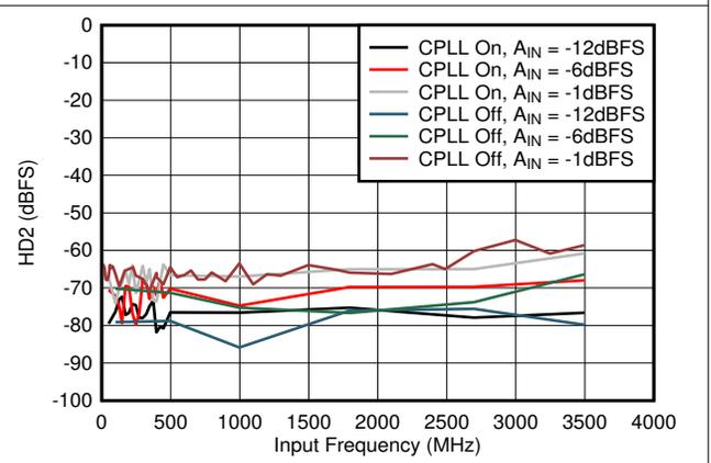
Figure 5-52. HD2 vs  $A_{IN}$  and C-PLL
