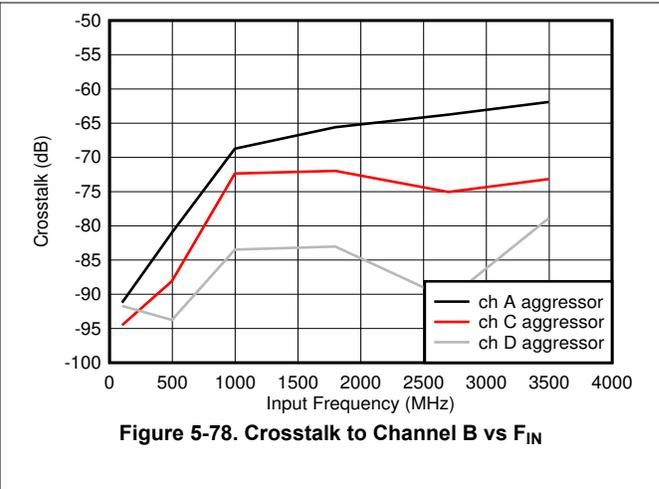
Figure 5-78. Crosstalk to Channel B vs  $F_{IN}$
