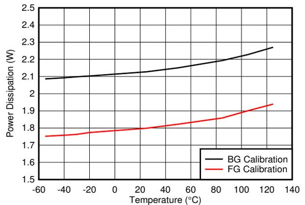
**Figure 5-122. Dual Channel, Power Dissipation vs Temperature**
