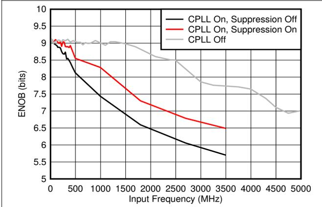
Figure 5-43. ENOB vs  $F_{IN}$  and C-PLL modes
