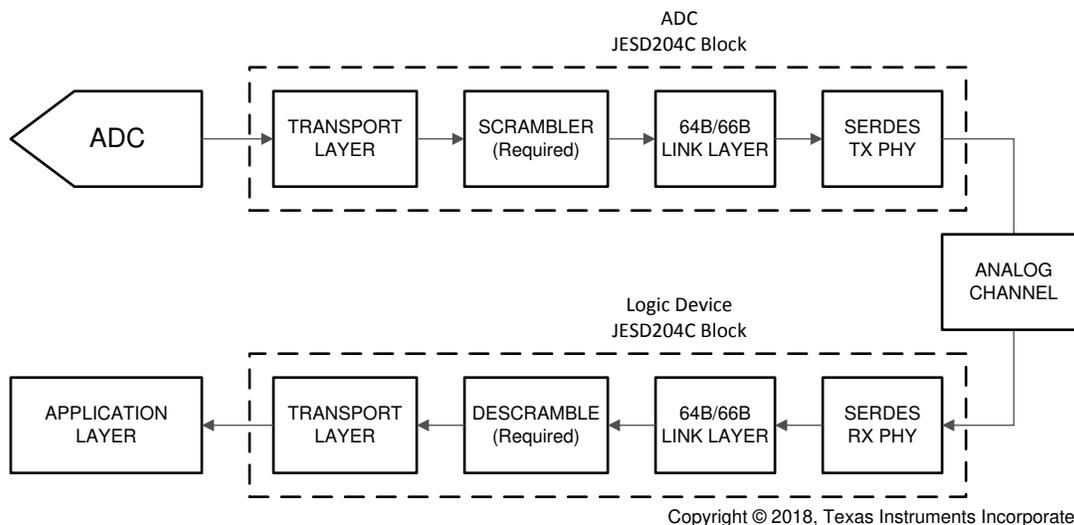
**Figure 6-6. Simplified 64B/66B Encoded JESD204C Interface Diagram**
