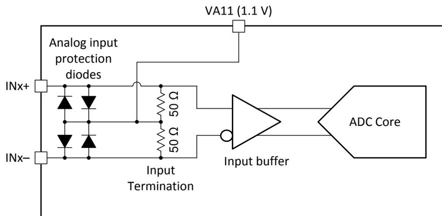
**Figure 6-2. Analog Input Internal Termination and Protection Diagram**
