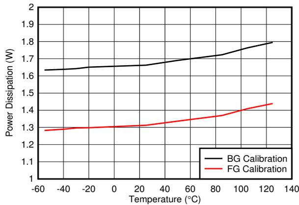
**Figure 5-123. Single Channel, Power Dissipation vs Temperature**
