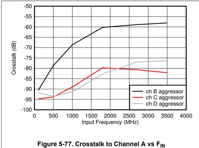
Figure 5-77. Crosstalk to Channel A vs  $F_{IN}$
