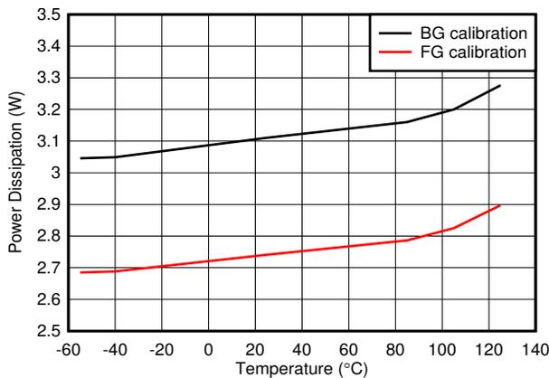
**Figure 5-121. Quad Channel, Power Dissipation vs Temperature**
