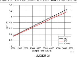
Figure 5-137. Dual Channel Mode: I<sub>VD11</sub> vs Sample Rate
