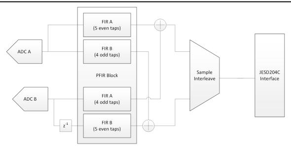
Figure 6-7. Alternate I/Q Correction-Type Filter Block Diagram
