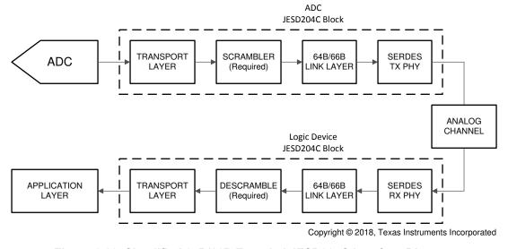
Figure 6-20. Simplified 64B/66B Encoded JESD204C Interface Diagram
