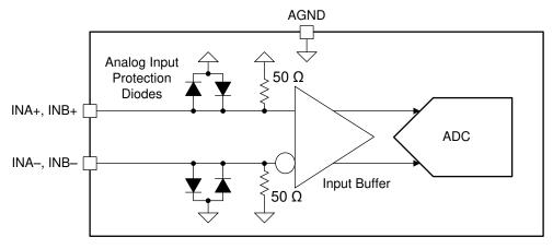
Figure 6-1. ADC12DJ5200-SEP Analog Input Internal Termination and Protection Diagram
