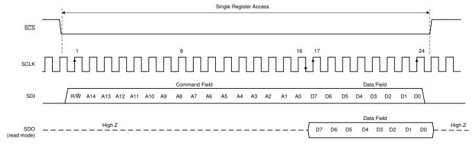
Figure 6-26. Serial Interface Protocol: Single Read/Write
