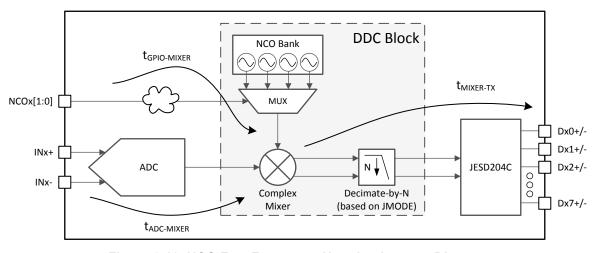
Figure 6-10. NCO Fast Frequency Hopping Latency Diagram
