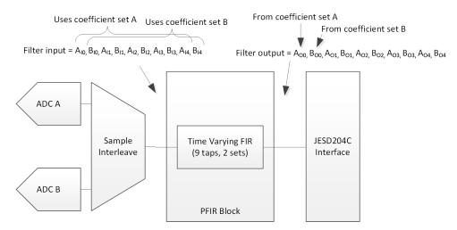
Figure 6-6. Time Varying Filter PFIR Block Diagram
