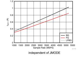
Figure 5-134. Dual Channel Mode: IVA11 vs Sample Rate
