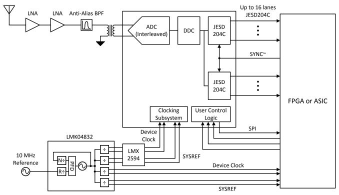
Figure 7-1. Typical Configuration for Wideband RF Sampling
