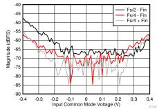
Figure 5-100. Fs/2 -  $F_{\rm IN}$  and Fs/4  $\pm$   $F_{\rm IN}$  vs Input Common Mode Voltage
