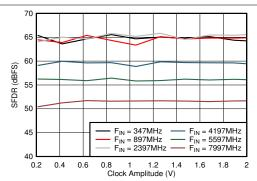
Figure 5-86. Dual Channel Mode: SFDR vs Clock Amplitude
