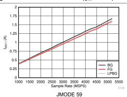
Figure 5-138. Dual Channel Mode: I<sub>VD11</sub> vs Sample Rate
