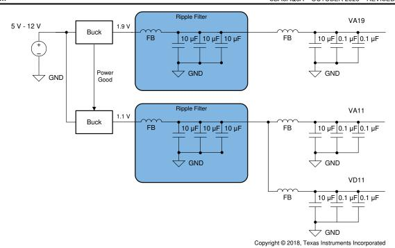
Ripple filter notch frequency to match the fs of the buck converter.
