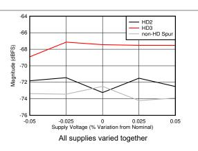
Figure 5-98. Dual Channel Mode: HD2, HD3 and Worst non-HD Spur vs Supply Voltage
