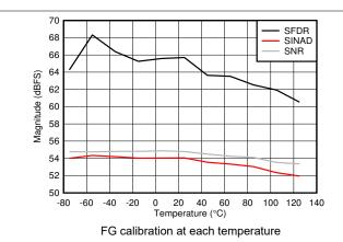
Figure 5-91. Dual Channel Mode: SNR, SINAD and SFDR vs
