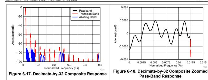
For maximum efficiency, a group of high-speed filter blocks are implemented with specific blocks used for each decimation setting to achieve the composite responses illustrated in Figure 6-11 to Figure 6-18. Table 6-13 describes the combination of filter blocks used for each decimation setting and Table 6-14 lists the coefficient details and decimation factor of each filter block. The coefficients are symmetric with the center tap indicated by bold text.
