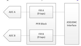
Figure 6-4. Dual Channel Equalization PFIR Block Diagram
