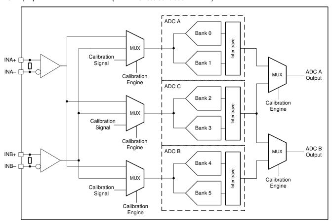
Figure 6-25. ADC12DJ5200-SEP Calibration System Block Diagram
