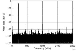
JMODE 1, FG calibration,  $f_S$  = 6400MSPS,  $f_1$  = 342MHz,  $f_2$  = 352MHz,  $A_{IN}$  = -7dBFS per tone, SFDR = -70dBFS, IMD3 = -91dBFS, IMD2 = -71dBFS
