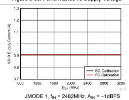
Figure 5-60. VA19 Supply Current vs Clock Rate
