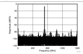
JMODE 3, FG calibration,  $f_S$  = 3200MSPS,  $f_1$  = 2477MHz,  $f_2$  = 2487MHz,  $A_{IN}$  = -7dBFS per tone, SFDR = -70dBFS, IMD3 = -74dBFS, IMD2 = -70dBFS
