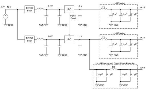
Figure 7-6. LDO Linear Regulator Example
