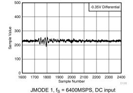
Figure 5-72. Background Calibration Core Transition (DC Signal Zoomed)
