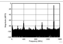
JMODE 3, FG calibration,  $f_S$  = 3200MSPS,  $f_1$  = 4992MHz,  $f_2$  = 5002MHz,  $A_{IN} = -7dBFS$  per tone, SFDR = -62dBFS, IMD3 = -63dBFS, IMD2 = -80dBFS
