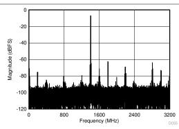
JMODE 1, FG calibration,  $f_S$  = 6400MSPS,  $f_1$  = 4992MHz,  $f_2$  = 5002MHz,  $A_{IN} = -7dBFS$  per tone, SFDR = -62dBFS, IMD3 = -65dBFS, IMD2 = -71dBFS
