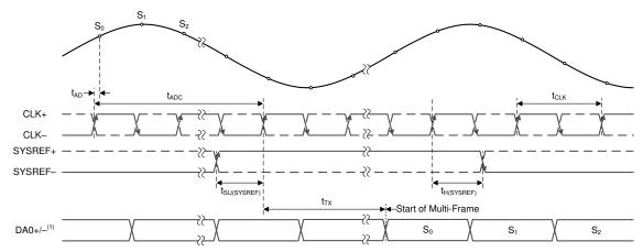
A. Only the SerDes lane DA0± is shown, but DA0± is representative of all lanes. The number of output lanes used and bit-packing format is dependent on the programmed JMODE value.
