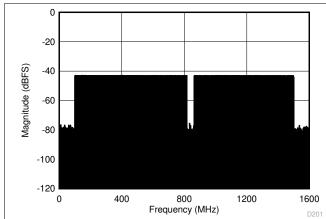
JMODE 3 ,  $f_S$  = 3200MSPS, signal band is 100MHz to 1500MHz, notch center frequency = 839.7MHz, notch bandwidth = 45MHz
