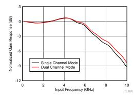
ADC12DJ3200QML-SP Measured Input Bandwidth
