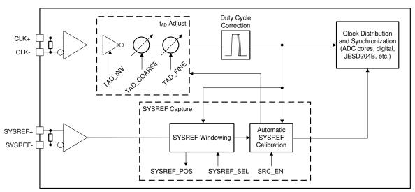
Figure 6-3. ADC12DJ3200QML-SP Clocking Subsystem
