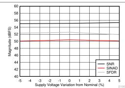
JMODE 1, FG calibration,  $f_S$  = 6400MSPS,  $f_{IN}$  = 2482MHz,  $A_{IN}$ = -1dBFS
