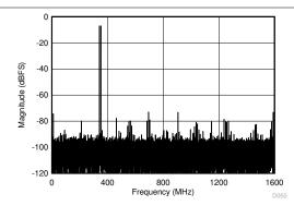
JMODE 3, FG calibration,  $f_S$  = 3200MSPS,  $f_1$  = 342MHz,  $f_2$  = 352MHz,  $A_{IN}$  = -7dBFS per tone, SFDR = -73dBFS, IMD3 = -87dBFS, IMD2 = -74dBFS
