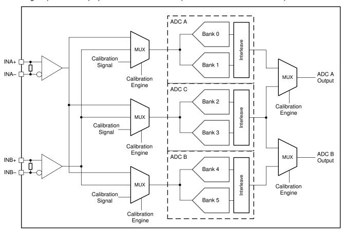
Figure 6-23. ADC12DJ3200QML-SP Calibration System Block Diagram
