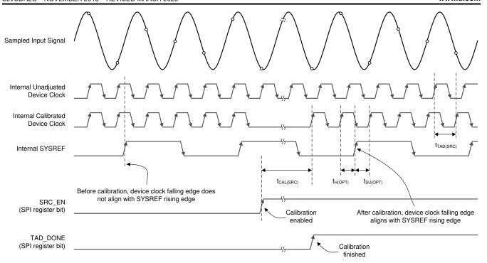
Figure 6-4. SYSREF Calibration Timing Diagram
