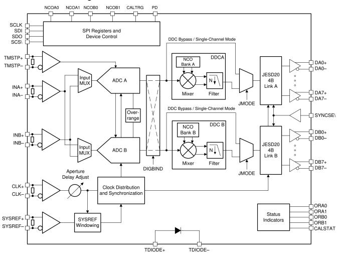
Figure 6-1. Functional Block Diagram
