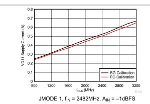
Figure 5-62. VD11 Supply Current vs Clock Rate
