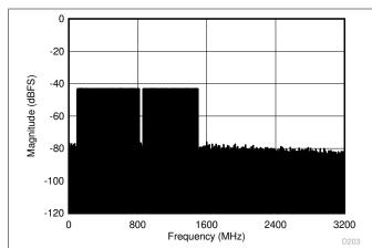
JMODE 1 ,  $f_S$  = 6400MSPS, signal band is 100MHz to 1500MHz, notch center frequency = 839.7MHz, notch bandwidth = 45MHz
