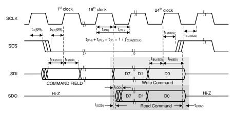
Figure 5-3. Serial Interface Timing
