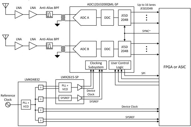
Figure 7-1. Typical Configuration for Wideband RF Sampling Receiver
