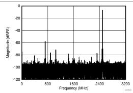
JMODE 1, FG calibration,  $f_S$  = 6400MSPS,  $f_1$  = 2477MHz,  $f_2$  = 2487MHz,  $A_{IN}$  = -7dBFS per tone, SFDR = -58dBFS, IMD3 = -70dBFS, IMD2 = -75dBFS
