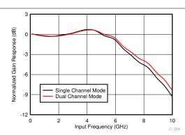
Figure 5-68. Gain Response vs Input Frequency
