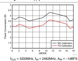
Figure 5-66. Power Consumption vs JMODE
