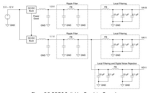
Figure 7-7. DC/DC Switching Regulator Example
