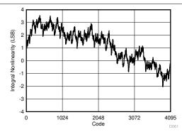
JMODE 1, FG calibration,  $f_S = 6400MSPS$ ,  $f_{IN} = 99.97MHz$
