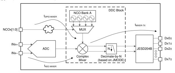
Figure 6-6. NCO Fast Frequency Hopping Latency Diagram
