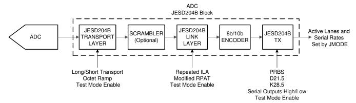
Figure 6-22. Test Mode Insertion Points
