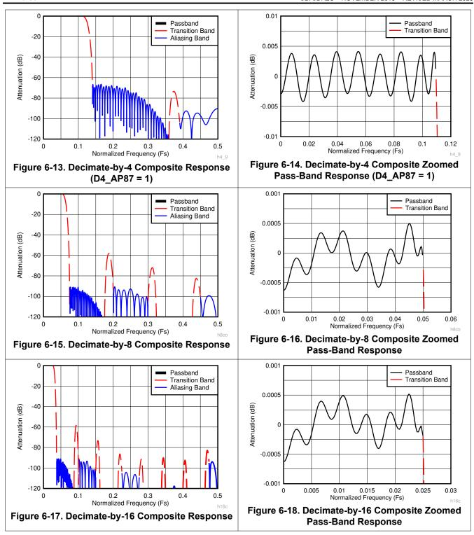
For maximum efficiency, a group of high-speed filter blocks are implemented with specific blocks used for each decimation setting to achieve the composite responses illustrated in Figure 6-7 to Figure 6-18. Table 6-11 describes the combination of filter blocks used for each decimation setting and Table 6-12 lists the coefficient details and decimation factor of each filter block. The coefficients are symmetric with the center tap indicated by bold text.
