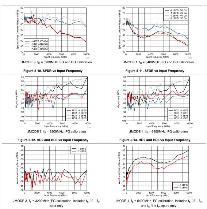
Figure 5-14. Worst Interleaving Spur vs Input Frequency
