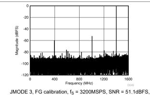
SFDR = 53dBFS, ENOB = 7.8 bits Figure 5-38. Single-Tone FFT at  $f_{\text{IN}}$  = 8197MHz,  $A_{\text{IN}}$  = -1dBFS
