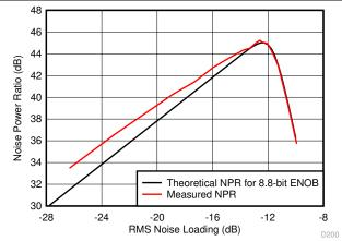
JMODE 3 ,  $f_S$  = 3200MSPS, signal band is 100MHz to 1500MHz, notch center frequency = 839.7MHz, notch bandwidth = 45MHz, peak NPR = 45.2dB at noise loading of -12.6dB
