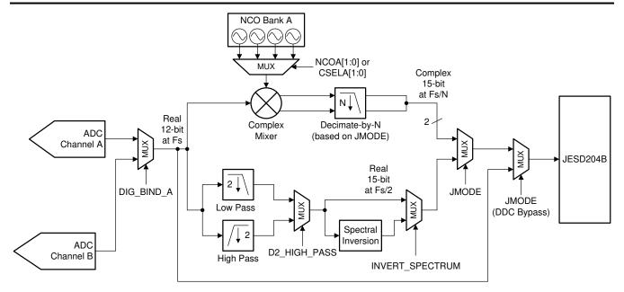
Figure 6-5. Channel A Digital Down Conversion Block (Dual-Channel Mode Only)
