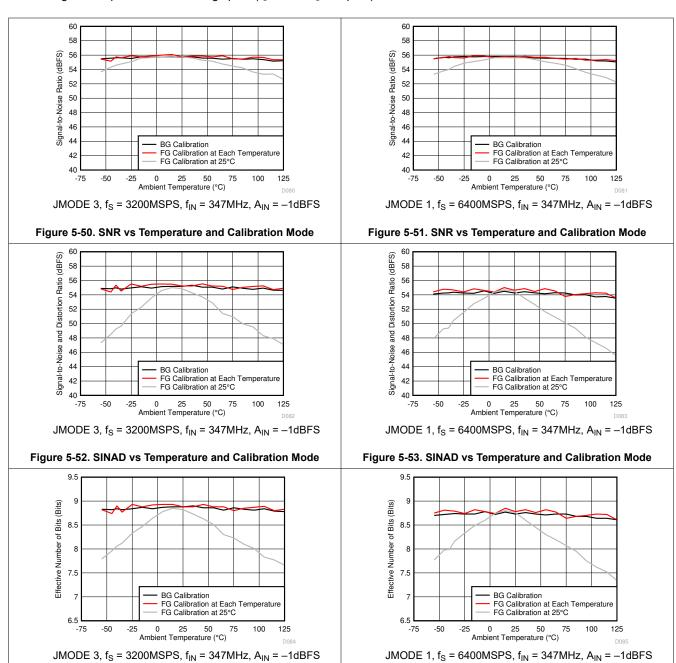
Figure 5-54. ENOB vs Temperature and Calibration Mode
