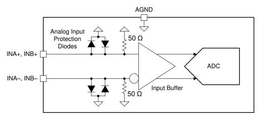
Figure 6-2. ADC12DJ3200QML-SP Analog Input Internal Termination and Protection Diagram
