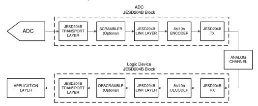
Figure 6-19. Simplified JESD204B Interface Diagram
