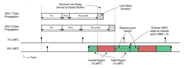
Figure 6-20. LMFC Valid Region Definition for Elastic Buffer Release Point Selection
