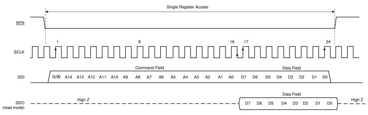
Figure 6-24. Serial Interface Protocol: Single Read/Write
