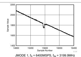
Figure 5-70. Background Calibration Core Transition (AC Signal Zoomed)
