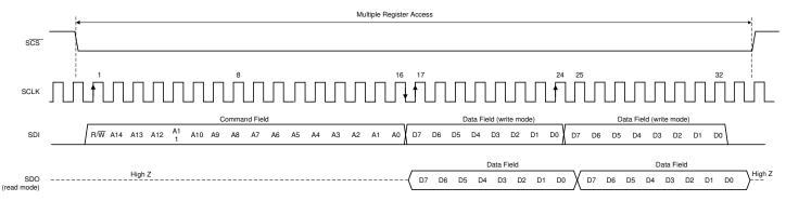
Figure 6-25. Serial Interface Protocol: Streaming Read and Write
