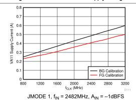
Figure 5-61. VA11 Supply Current vs Clock Rate
