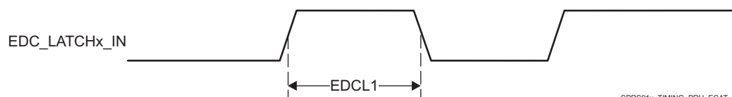
Figure 5-69. PRU-ICSS ECAT LATCHx_IN Timing
